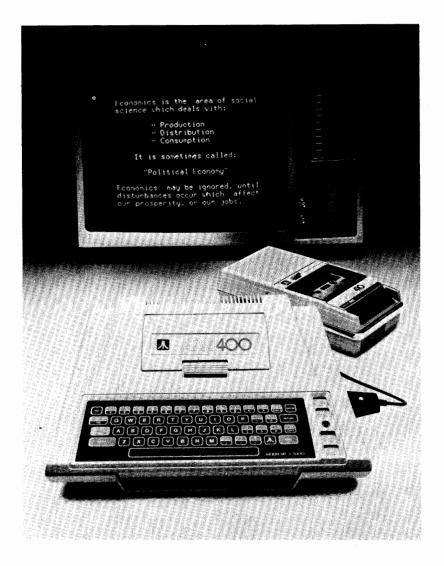
The Atari 400 computer. This personal computer system uses a cassette tape recorder as external storage. The CRT is a special unit providing both capital and lower-case letters in a large dot-matrix system. Photo courtesy of Atari Computers
