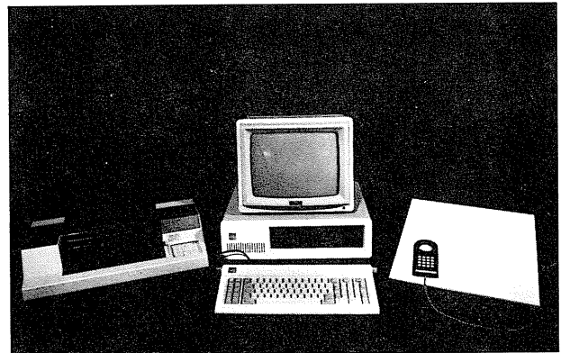
It adds $3000-4000 to the price of an IBM PC, but jazzing up the desktop micro with specialized drawing equipment turns it into a full-fledged CAD system. This photo shows a typical configuration: IBM PC plus a $1400 GTCO digitizing tablet (precision input), $1290 MicroVitec CUB graphics monitor (high-resolution screen display) and a $1095 Hewlett-Packard 7470-A plotter (high-resolution output).
