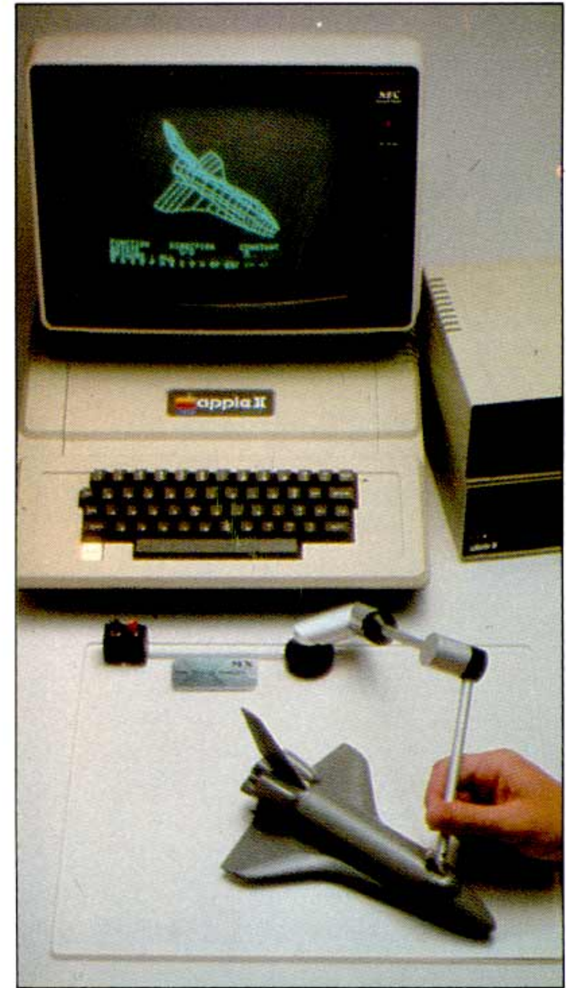
With the ADVANCED SPACE GRAPHICS hardware/software combination you can trace a physical object in 3-D on the screen by moving the "Space Tablet" around the object's surface.
