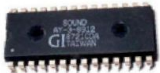
» Talk about a song and dance... The AY chip that generated the exciting new Speccy sound.
