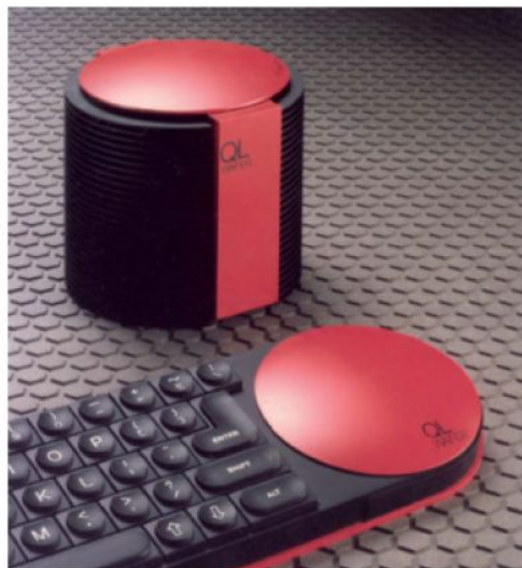
» Beyond the QL... Rick Dickinson's prototype design for the QL Plus, with built-in wafer drive and accompanying wafer stack. The design never progressed beyond this model.
