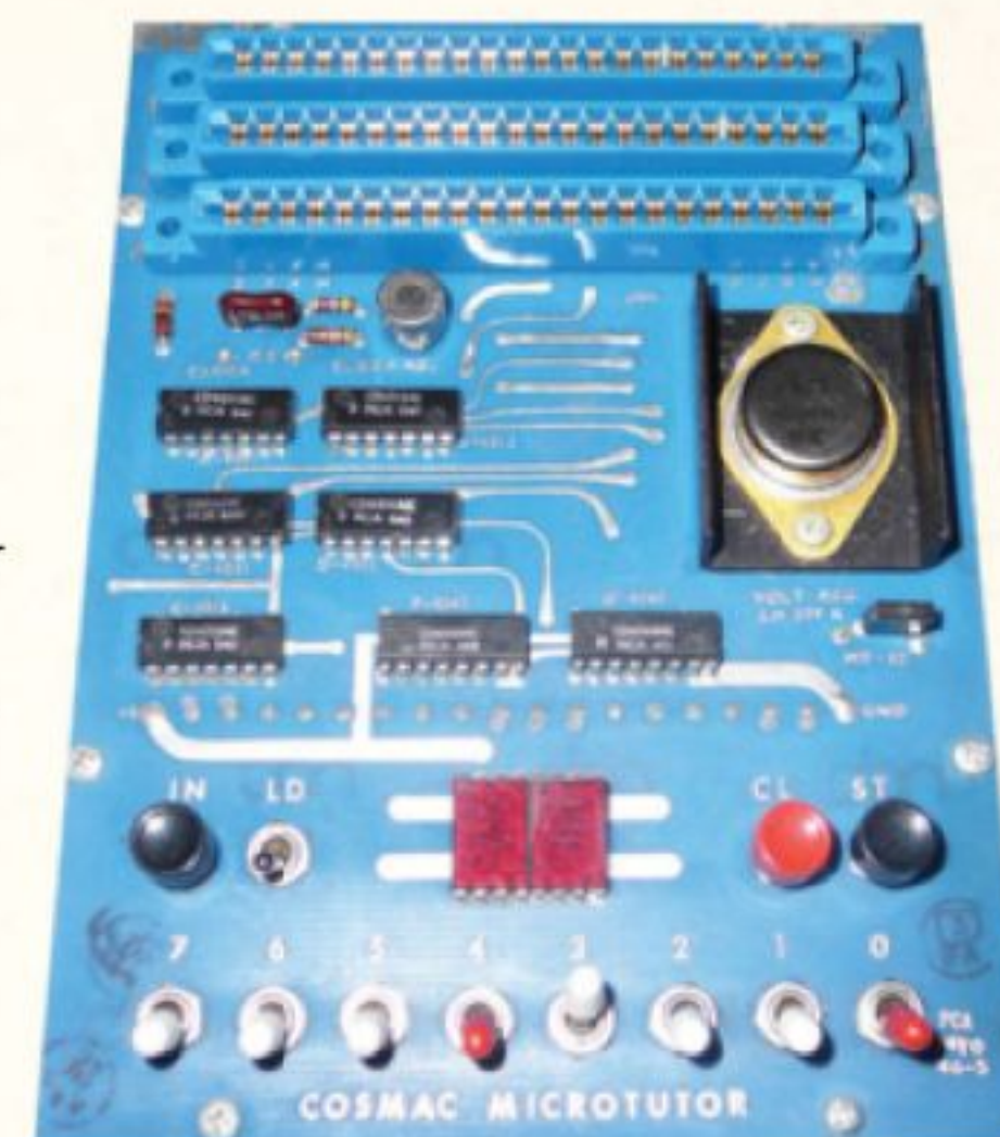
» An impressive closeup of the COSMAC Microtutor main unit. The main processing parts are on removable cards that dock in the empty slots shown.
