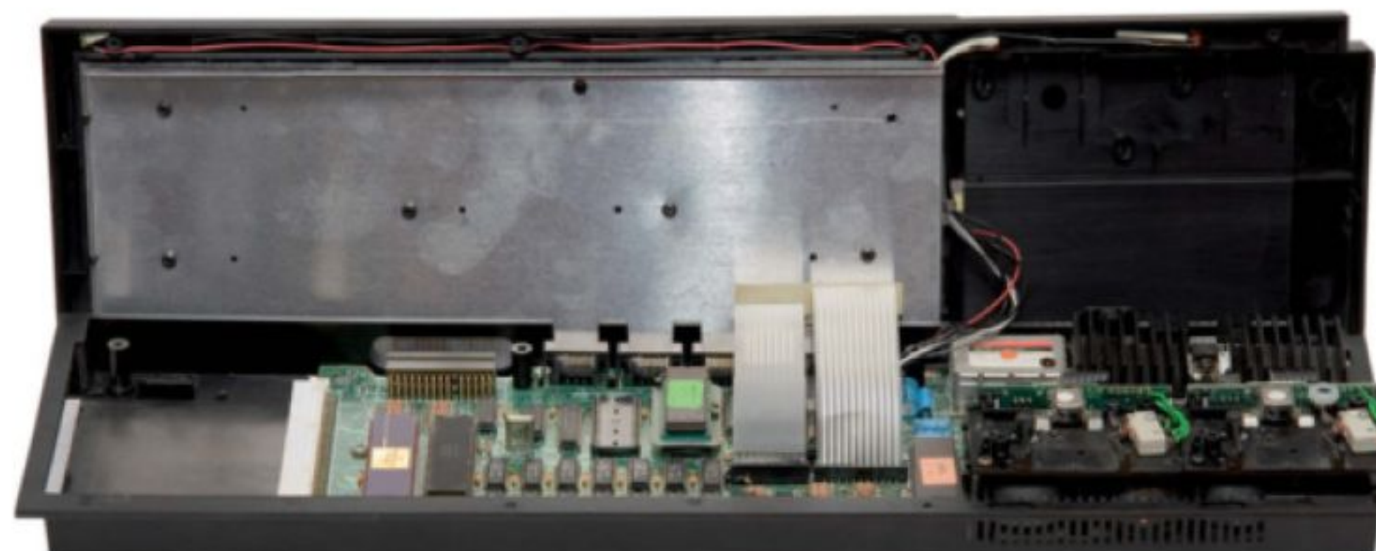
» Under the hood: the empty space on the left was an expansion bay for housing additional memory and peripherals.
