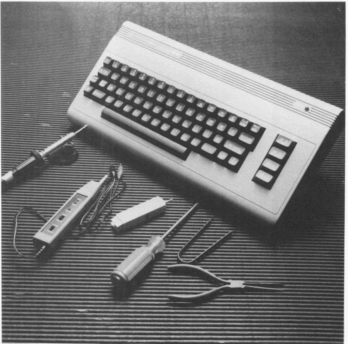
Fig. 2-1. The 64's case can be opened with a Phillips head screwdriver. The print board is removed with the aid of a soldering iron and longnose pliers.
