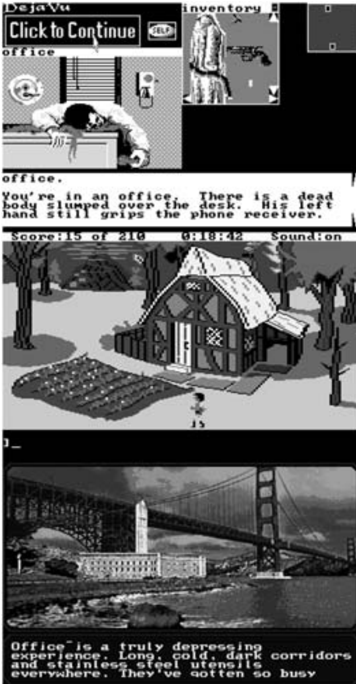
Figure 15.1 Examples of different graphics standards: CGA (top), EGA (center), and VGA (bottom). Even in these black and white reproductions, differences in spatial resolution and color resolution show the improvements from one standard to another.
