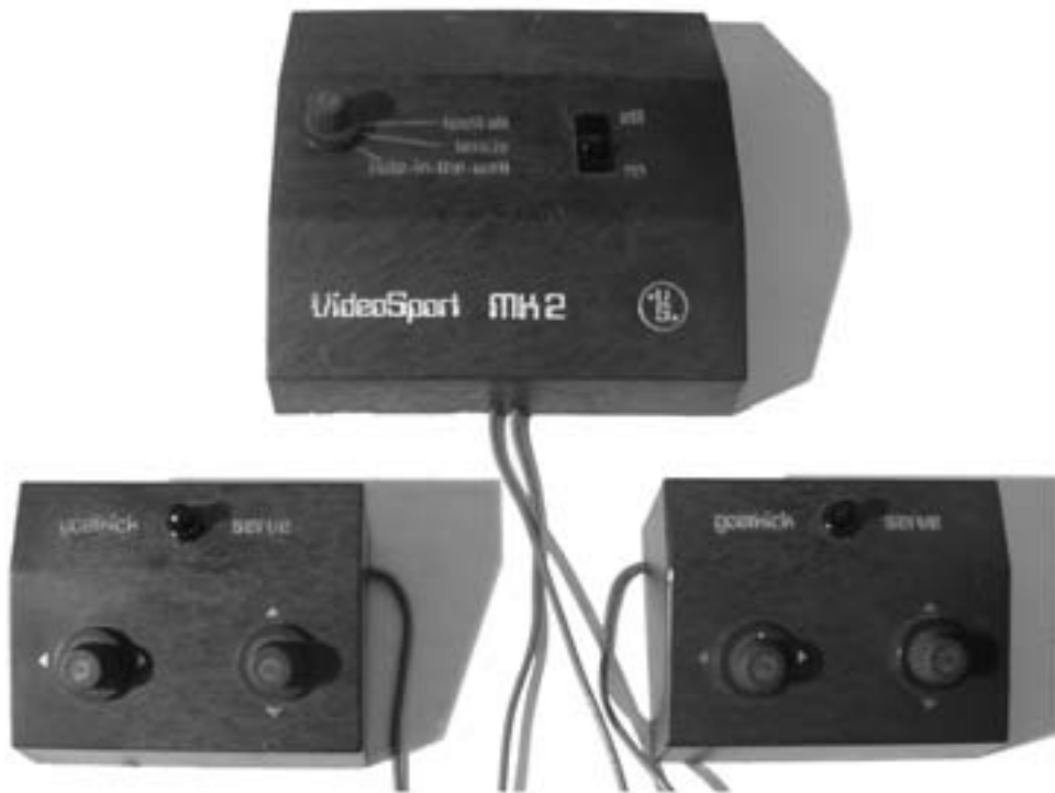
Figure 8.4 The VideoSport MK2. Advertised by Henry's in early 1975 in England, the VideoSport MK2 is believed to be the second oldest system from the United Kingdom and remains one of the earliest European games after the first Videomaster Home T.V. Game (1974–1975). Almost entirely analog, it uses discrete components and only two very simple chips.
