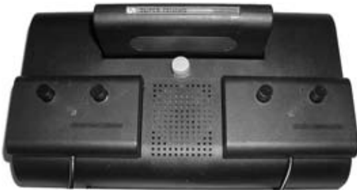
Figure 8.2 Interton Video 2000 (Germany, 1975). The first ball-and-paddle game to use cartridges after the Magnavox Odyssey, the Interton Video 2000 used discrete components and several logic gates; it had no dedicated chips and no processor. Only five cartridges were designed for it. This system also was cloned in Spain around 1976 under the TeleTennis name.
