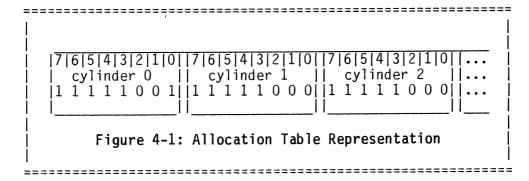
A 5-1/4" single density diskette is formatted at ten sectors per track, five sectors per granule, two granules per track. A two-sided diskette has twice the number of granules per track available on each cylinder. Thus, the single density single, sided 5-1/4" configuration will use only bits 0 and 1
