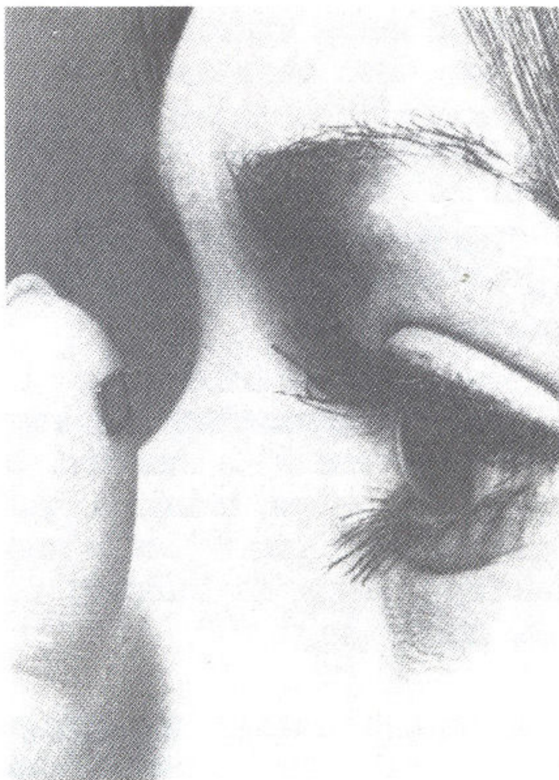
The tiny chip of silicon on the girl's finger is a microprocessor which contains the equivalent of 20,000 transistors.
