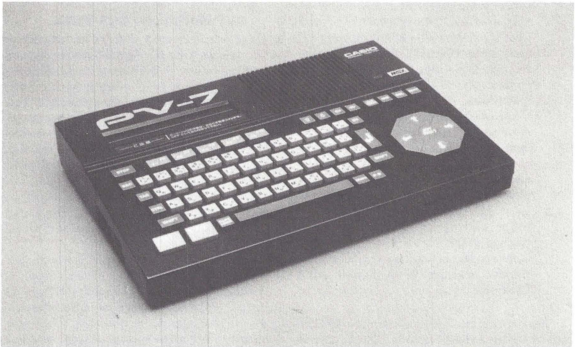
Fig. 3-1. Casio has designed some MSX computers for light weight and low manufacturing cost. They lack some of the features of more expensive models (courtesy of Microsoft Corp.).
