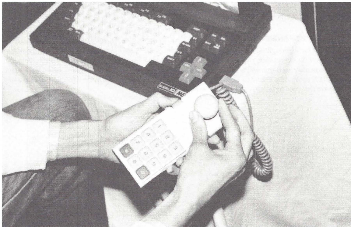
Fig. 4-2. A Coleco joystick can be readily used with an MSX computer, although the number pad will not function.
