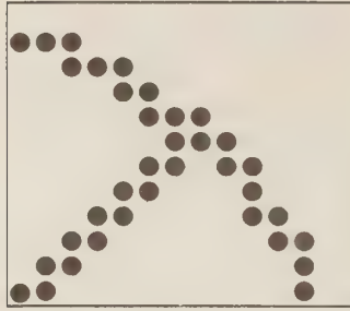
FIG. 20-8 Use of clipping to select part of an enlarged image of a wheel
