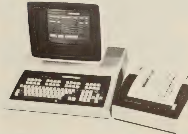
FIG. 22-33 Thermal printer used to record the display of a video monitor
