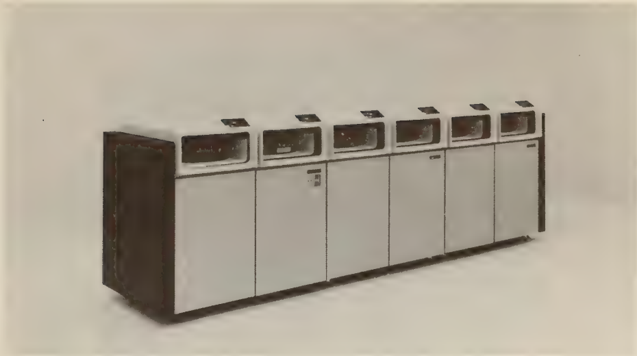
FIG. 2-6 Magnetic disk storage (IBM Corp. Ltd.)
