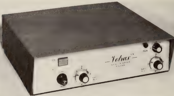
FIG. 29-9 The Votrax model VS-6 electronic voice system speech synthesizer (Votrax Division of Federal Screw Works)
