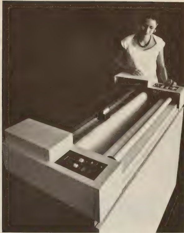
FIG. 23-8 A free-standing four-pen drum plotter with a plotting area 34 in (864 mm) wide by the length of the paper roll (California Computer Products, Inc.)
