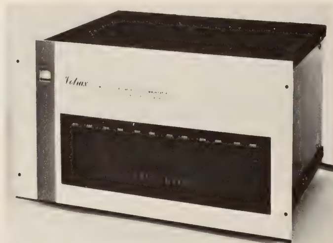
FIG. 29-1 An audio-response unit containing 128 s of speech stored in digital form (Votrax Division of Federal Screw Works)
