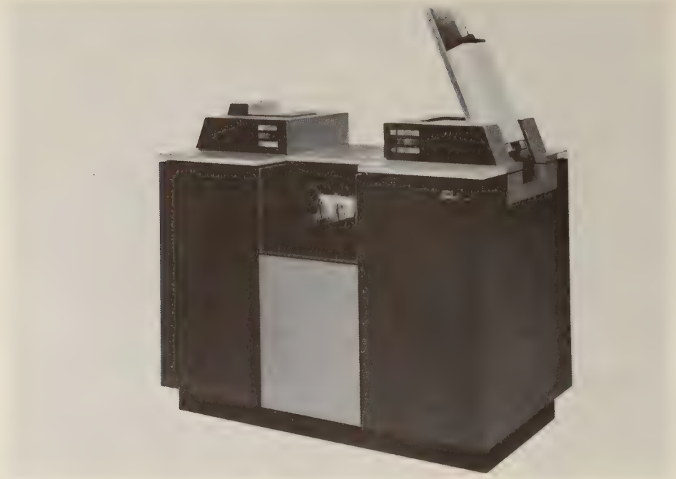
FIG. 2-5 A punched card reader (IBM Corp. Ltd.)
