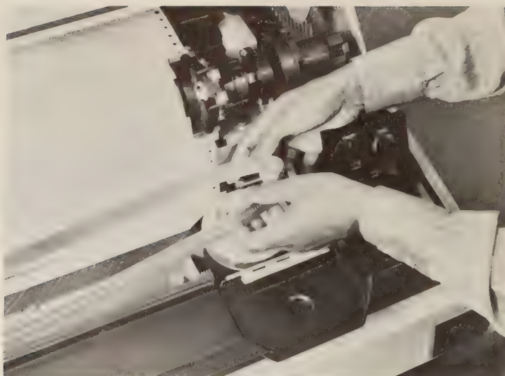
FIG. 22-10 The print band on this band printer is easily changed to permit substitution of character sets (Dataproducts Corp.)
