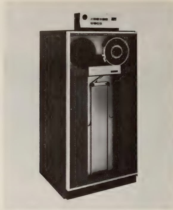
FIG. 2-7 A magnetic tape unit (IBM Corp. Ltd.)
