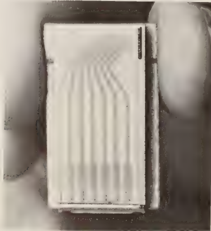
FIG. 22-31 Thermal dot-matrix print head for printing a character at a time (Dataproducts Corp.)
