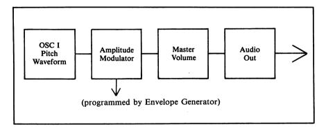
This is the basic format for programming a sound. Adding filters and ring modulators is like icing on the cake. We'll get to them later. For now, let's take a more in-depth look at how to program these main controls, which are the primary ingredients in our sound recipe.
