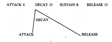
Combined with the proper waveform, pitch range and sometimes with the help of filters, the ADSR plays a big role in the total sound produced.
