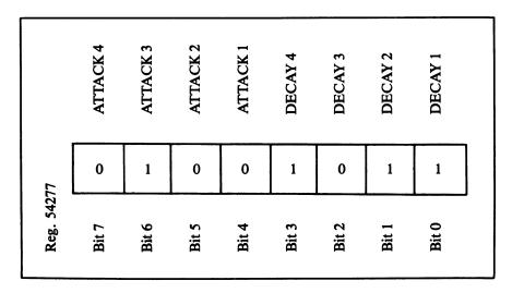
That's because the decimal number 75 is the same as the binary number Ø1ØØ1Ø11. In this manner, our statement POKE 54277,75 turns on DECAY bits Ø, 1, 3 and ATTACK bit 6, giving us a combination of three DECAY settings and one ATTACK setting. So you see, our number 75 does a lot of work.
