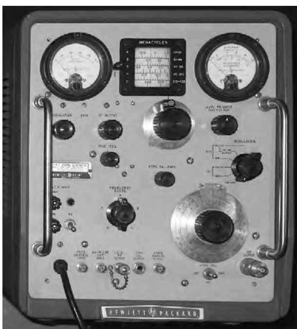
Fig 25.37 — A classic Hewlett-Packard 608F tube-type signal generator. While not as stable as modern synthesized signal generators, in other respects the performance is quite up to date.
