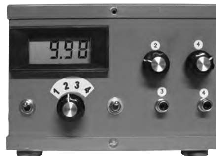
Fig 7.55 — The front panel of the four-output switching supply.
