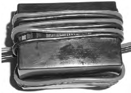
Fig 21.85 — RF choke for screwdriver antenna control and power leads.
