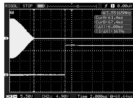
Fig 24.70 — The same ICOM IC-7200 timing from RF-stop to relay contacts open. There is 6 ms between the end of the RF output and the relays returning to receive.
