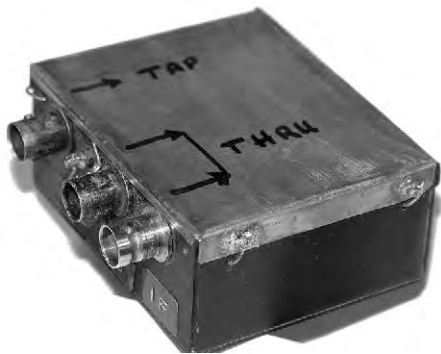
Fig 13.61 — Sample of a box made with PC board with a sheet brass cover overlapping all four sides. Note the BNC connectors and feed thru insulator.
