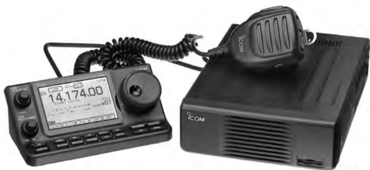
Fig 6 — The Icom IC-7100 desktop HF, 6 and 2 meter and 70 cm transceiver. This radio offers a convenient angled front panel for desk or vehicle use and is the first with a touch screen,
