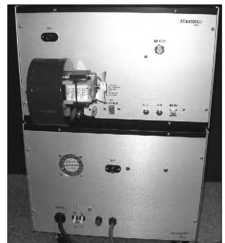
Fig 17.56 — At the top, front panel view of RF Deck and Power Supply for 3CX1500D7 amplifier. At bottom, rear view of RF Deck and Power Supply.
