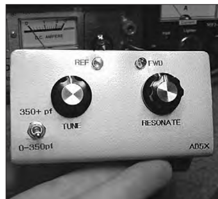
Fig 24.1 — The Z-Match Tuner handles 100 W and can be used from 80 through 10 meters.
