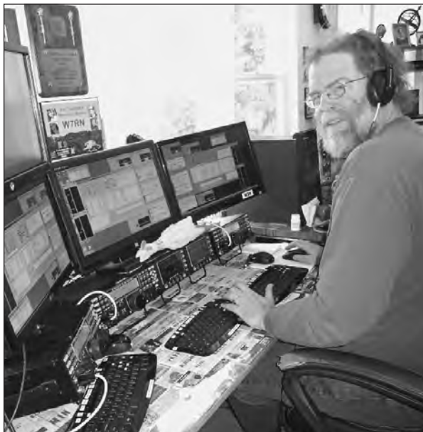
Fig 1.13 — Ham radio contesting or "radiosport" attracts thousands of participants. Jeff Stai, WK6I, took advantage of modern computer technology to set a West Coast record score in the 2013 ARRL RTTY (radioteletype) Roundup event. RTTY (pronounced "ritty" by most hams) is a keyboard-to-keyboard mode. Computer software and displays have taken the place of old-fashioned electromechanical teleprinters as well as paper logbooks. A computer also controls his radio. [Tom Taormina, K5RC, photo]
