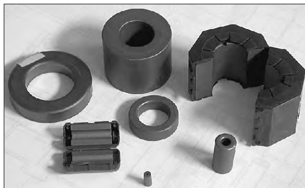
Fig 5.44 — Ferrites are made in many forms. Beads are cylinders with small center holes so that they can be slid over wires or cables. Toroidal cores are more ring-like so that the wire or cable can be passed through the center hole multiple times. Snap-on or split cores are made to be clamped over cables too large to be wound around the core or for a bead to be installed.
