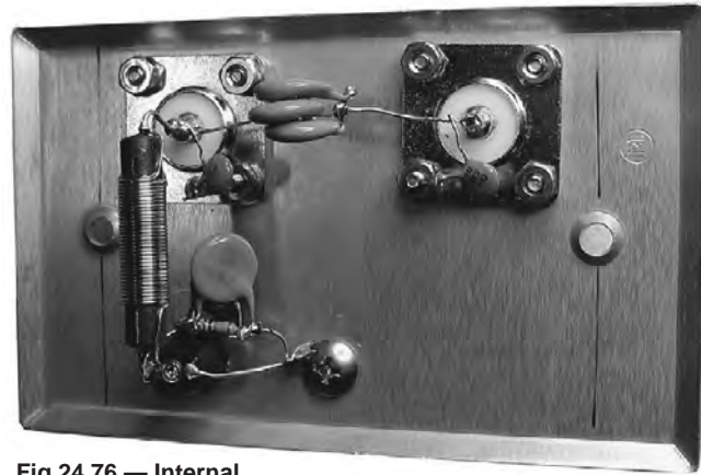
Fig 24.76 — Internal construction of the bias-Tee, following good RF construction practices.
