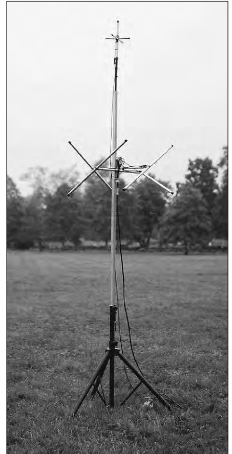
Fig 52 — The EZ-Lindenblad as a portable or Field Day antenna. A 70 cm antenna is on the top.
