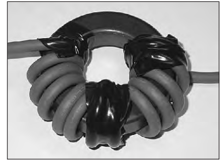
Fig 5.50 — A ferrite choke consisting of multiple turns of cable wound on a 2.4-in. OD x 1.4-in. ID x 0.5-in. toroid core.
