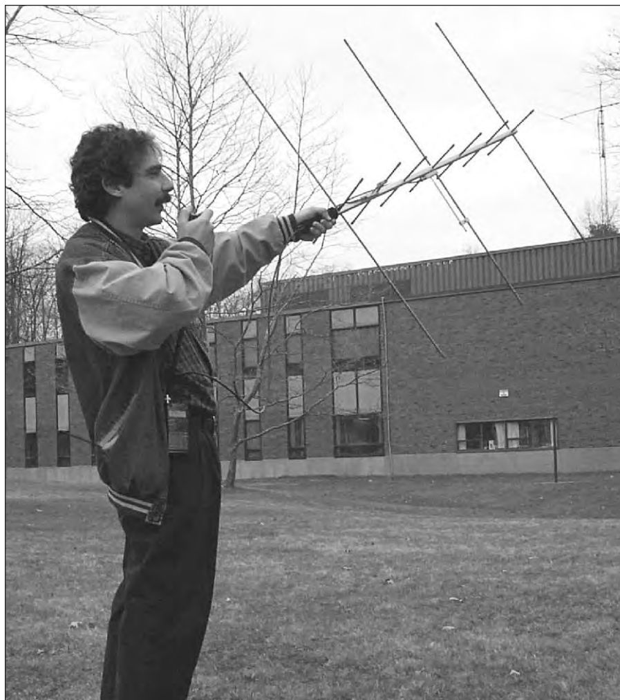
Fig 18 — Joe Bottiglieri, AA1GW, uses a dual-band Yagi to work a low-Earth orbiting FM repeater satellite with a handheld transceiver.
