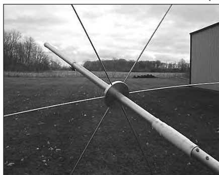
Fig 21.48 — The completed capacitance hat assembly is shown at A, and B shows a view of the upper mast assembly with the loading coil and capacitance hat.
