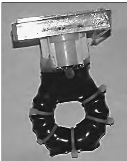
Fig 25.70 — Assembly of the RF current probe. Use an all-plastic meter and mount the circuits and toroid directly on the back of the meter case.
