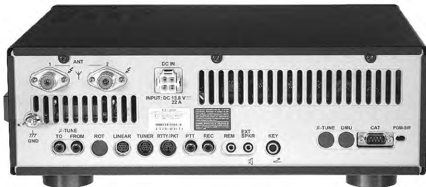
Fig 29.10 — The back of this Yaesu FT-950 transceiver shows some of the many types of connectors encountered in the amateur station. Note that this variety is found on a single piece of equipment.
