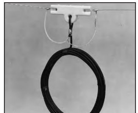
Fig 20.24 — RF choke formed by coiling the feed line at the point of connection to the antenna. The inductance of the choke isolates the antenna from the outer surface of the feed line.
