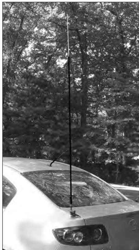
Fig 21.82 — Continuously-loaded whip antennas are short and lightweight. The base section consists of a fiberglass tube wound with wire to form the loading inductor. At the top of the base section the length of a steel whip or stinger can be adjusted to bring the antenna to resonance. [Joel Hallas, W1ZR, photo]
