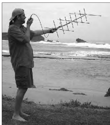
Fig 1.23 — Hams can use simple antennas and hand-held radios to contact amateur satellites, even the International Space Station. Sean Kutzko, KX9X took his satellite gear along during a vacation to Puerto Rico, making contacts via the AO-27 orbiting "bird." [Ward Silver, (NØAX, photo)]
