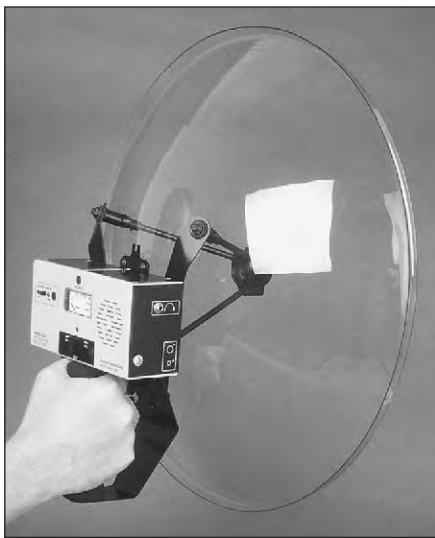
Fig 27.10 — The clear plastic parabolic dish is an “ear” connected to an ultrasonic detector that lets utility personnel listen for the sound of arcs.
