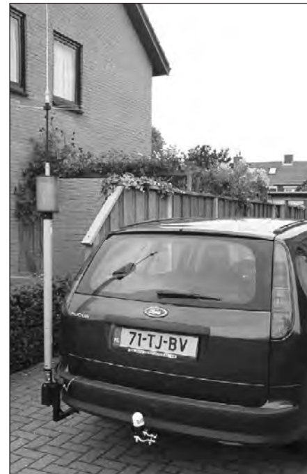
Fig 21.89 — The PA3VOS antenna mount easily supports a large screwdriver antenna and is offset to allow the hatch to open and close without removing the antenna.
