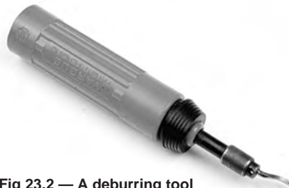
Fig 23.2 — A deburring tool is used to remove the burrs left after drilling a hole.
