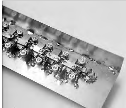
Fig 25.74 — The attenuator before final mechanical assembly. The 1/4-inch strips are spaced 0.033 inch apart to form a 50- \Omega connection from the BNC connector to the stripline. There are 1/2-inch square shields between 10-dB sections. The square shields have a notch in one corner to accommodate the end of the rectangular tubing.
