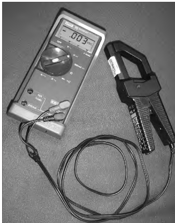
Fig 26.2 — A clamp-on meter probe is used with a digital multimeter for measuring ac current (left). Meters are also available integrated with the clamp-on probe (right).
