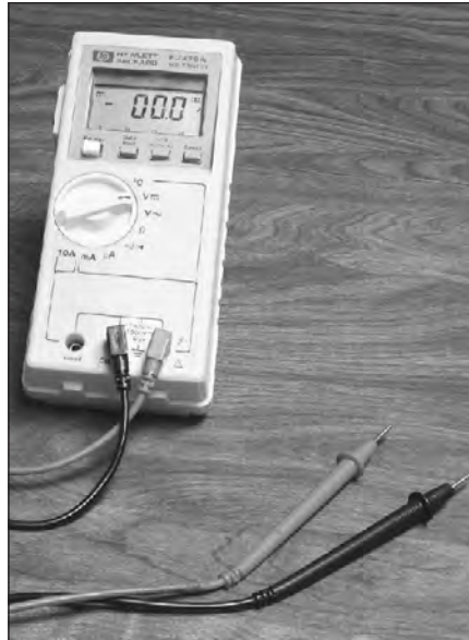
Fig 25.4 — A modern digital multimeter typically has a liquid crystal display readout.
