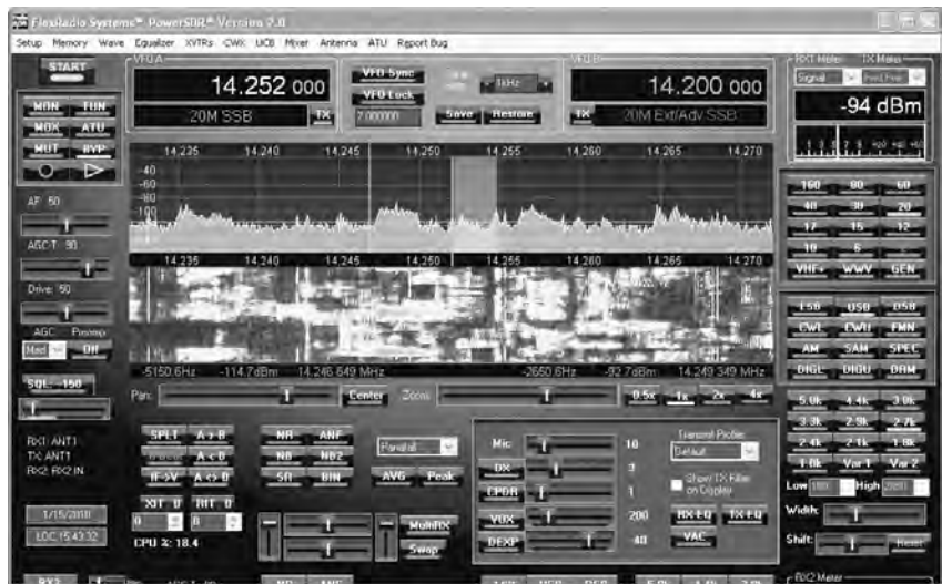
Fig 26 — One version of the main operating screen of PowerSDR operating software.
