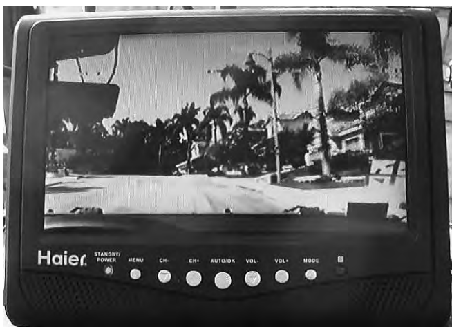
Fig 18 — Mobile ATV as shown here with a portable TV works fine using D-CATV 64-QAM, but it exhibits occasional freeze or tile effect from drop outs and multipath.
