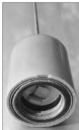
Fig 21.93 — The NMO (New Motorola) mount is widely used for VHF and UHF mobile antennas. It is available in mag-mount, trunk and lip mount and through-body mounting styles.
