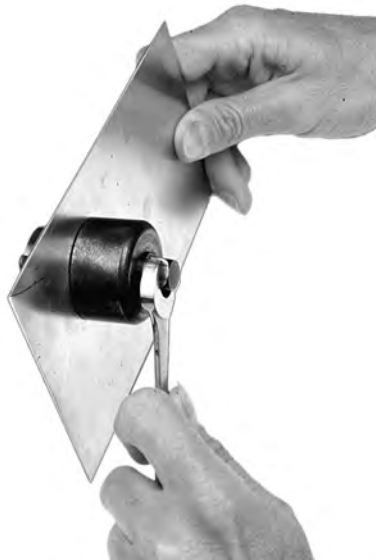
Fig 23.3 — A socket punch is used to punch a clean, round hole in sheet metal.
