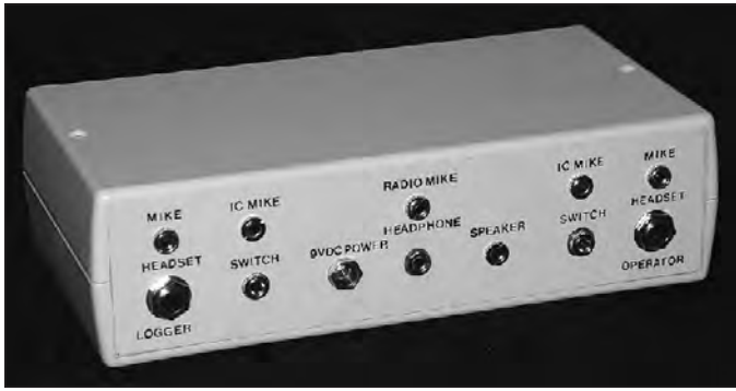
Fig 24.65 — Rear view of the audio interface box. Operator jacks are on the right, logger on the left. Connections to the radio are in the center.
