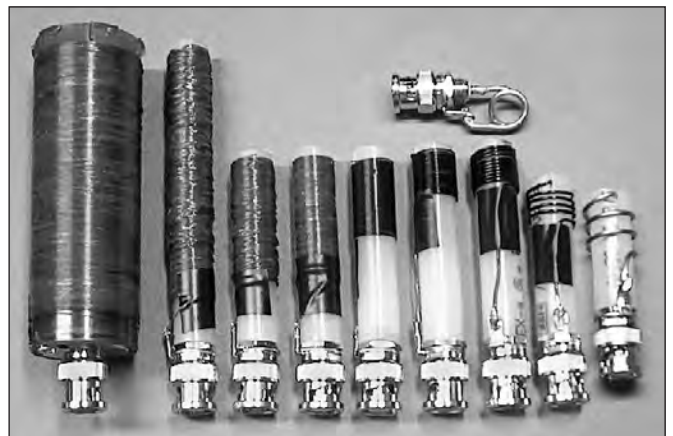
Fig 25.82 — This is how the coils look before covering them with heat-shrink tubing or tape. Small pieces of electrical tape are used to hold the turns in place during construction.
