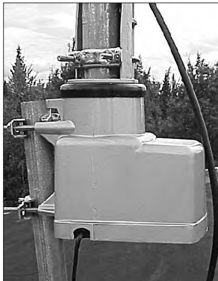
Fig 26 — A basic antenna rotator; the light-duty variety used to turn TV antennas. The wire exiting the bottom of the rotator housing is the multiconductor cable responsible for power and control.
