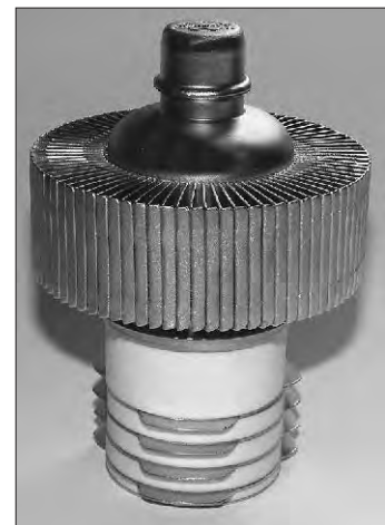
Fig 17.9 — Modern power tubes, such as this 4CX1000A tetrode, tend to use metal and ceramic construction.
