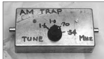
Fig 11.79 — The wave trap can be roughly calibrated to indicate the frequency to which it is tuned.
