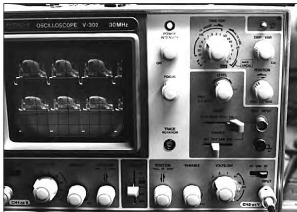
Fig 13 — An oscilloscope used to observe a video waveform. The lower trace is the video signal as it comes out of the sync stretcher. The upper trace is the detected RF signal from the amplifier.
