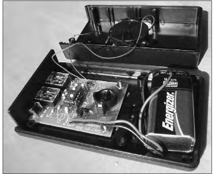
Fig 24.53 — The enhanced EMB version of the TiCK-4 includes a low-current regulator, battery backup and board-mounted jacks and switches.
