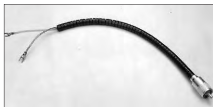
Fig 20.30 — W2DU bead balun consisting of 50 FB-73-2401 ferrite beads over a length of RG-303 coax. See text for details.
