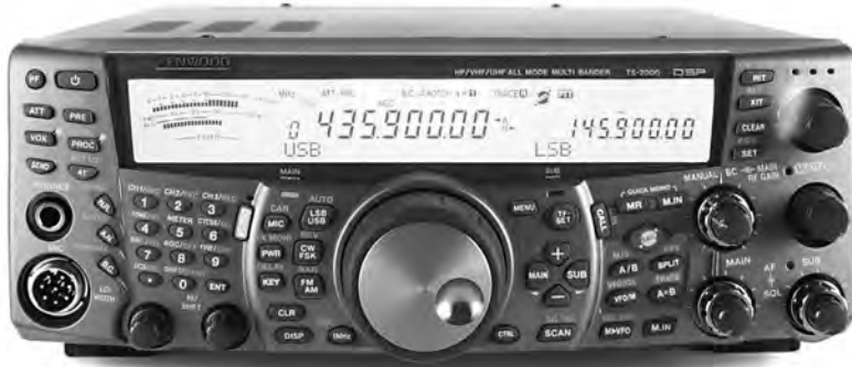
Fig 10 — Kenwood TS-2000. This transceiver operates on MF, HF, VHF, UHF, and the 1.2 GHz band as an option, providing broad frequency coverage in a single package.
