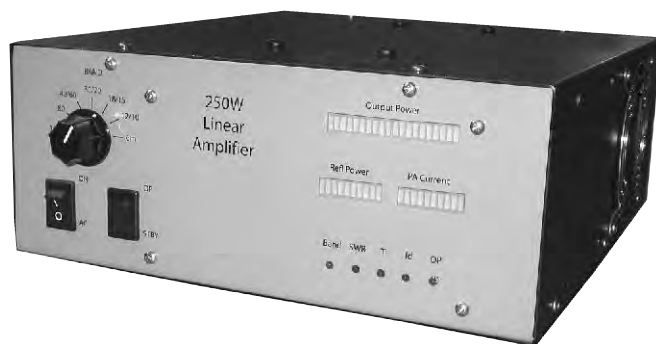
Fig 17.44 — This 250 W amplifier for 160 through 6 meters provides a detailed design example as well as a practical project. Additional photos and information about the interior layout may be found on the Handbook CD-ROM.
