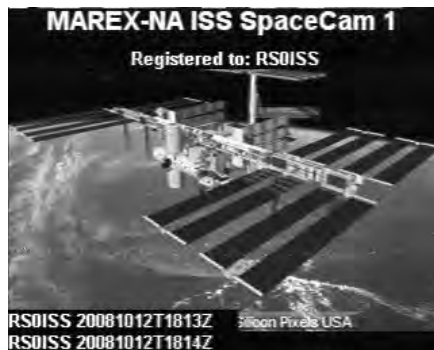
Fig 35 — Color SSTV image received from the International Space Station in Martin 1 mode 10/12/08 on 145.800 MHz FM.
