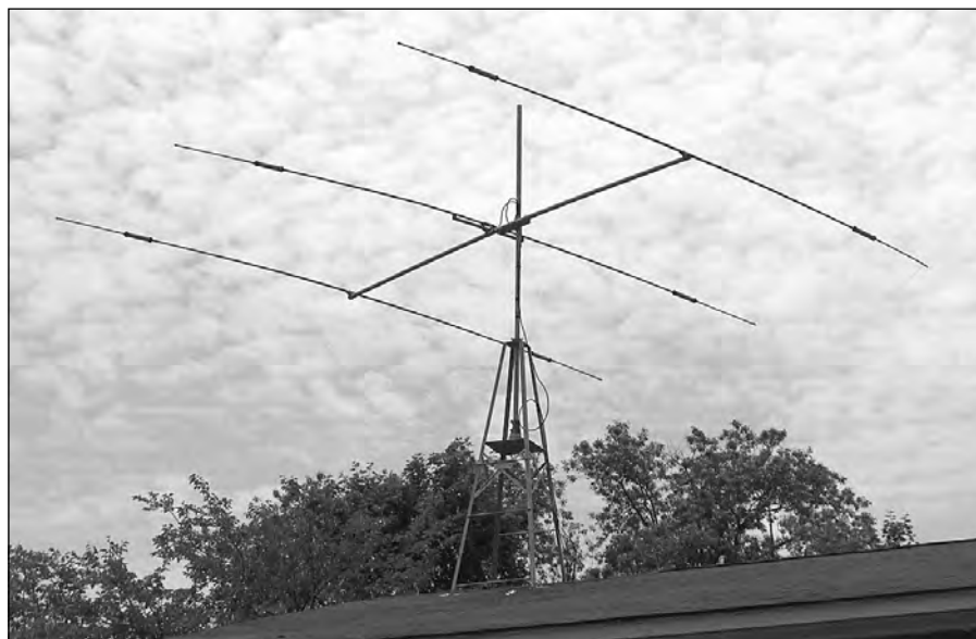
Fig 28.12 — The roof-mounted tower holding the AA2OW antenna system. (AA2OW photo)
