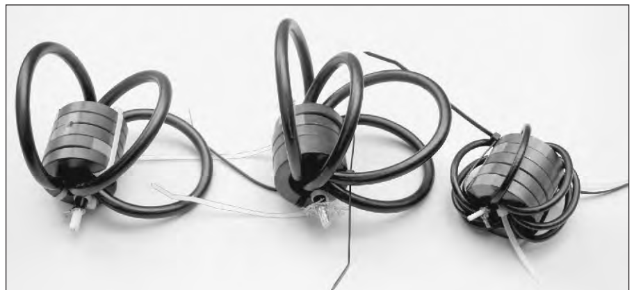
Fig 20.26 — Typical transmitting wound-coax common-mode chokes suitable for use on the HF ham bands.
