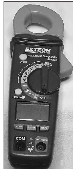
Fig 26.2 — A clamp-on meter probe is used with a digital multimeter for measuring ac current (left). Meters are also available integrated with the clamp-on probe (right).
