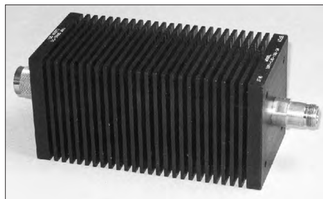
Fig 25.39 — A 100-watt power attenuator rated for dc-3000 MHz. The transmitter is connected to the male type-N connector. The female connector is for the low-power connection.
