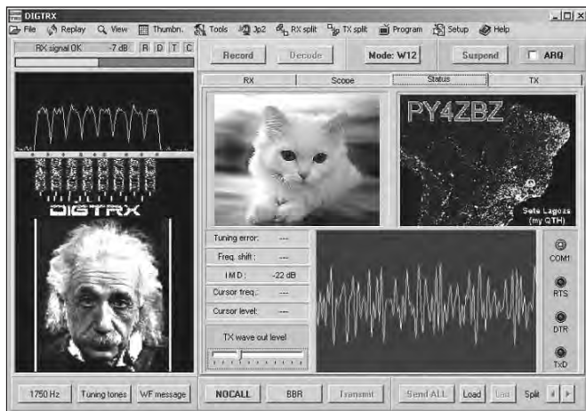
Fig 1.17 — Slow-scan television (SSTV) allows hams to exchange pictures over the air without wide-bandwidth live video equipment.
