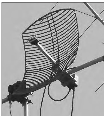
Fig 25 — The 2.4 GHz satellite downlink antenna at ARRL Headquarters station W1AW is a so-called “barbecue grill” dish antenna originally designed for the Multichannel Multipoint Distribution Service (MMDS). These inexpensive antennas can be assembled and installed in minutes.
