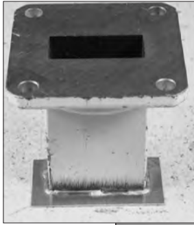
Fig 23.29 — Larger assemblies may be soldered with a heat gun. A torch is better for high-temperature brazing.
