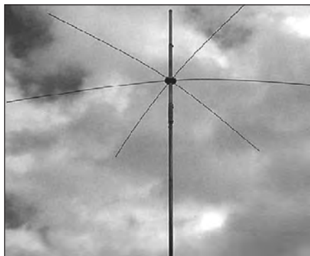
Fig 21.47 — W9SR's short vertical uses top loading and a capacitance hat with a 10 foot TV mast to make a compact antenna for 160, 80 or 40 meters.
