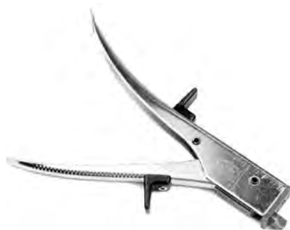
Fig 23.1 — A nibbling tool is used to remove small sections of sheet metal.
