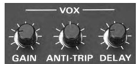
Fig 13.50 — The function of VOX controls is described in the text. They require adjustment for different types of operating, so front-panel knobs make the most convenient control arrangement. In some radios, VOX settings are adjusted through the menu system.
