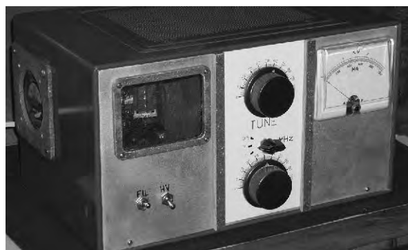
Fig 17.53 — The front panel of the Everyham's Amplifier. This version is designed to cover three bands (80, 40, and 20 meters). A window is included at left to allow viewing of the tube.
