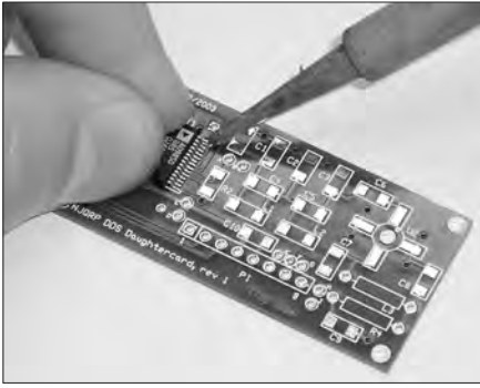
Fig 23.7A — This DDS Daughtercard has all interconnections on the top side. Connections to the ground plane on the backside of the board are made by the use of “vias,” wires through the PC board. Pin 28 of the SMT IC is shown being tack-soldered to hold it to the board, keeping all other pins carefully aligned on their pads. Then the other pins are carefully soldered, starting with pin 14 (opposite pin 28). Finally, pin 28 is reheated to ensure a good connection there. If you bridge solder across adjacent pads or pins, use solder wick or a vacuum solder sucker to draw off the excess solder.
