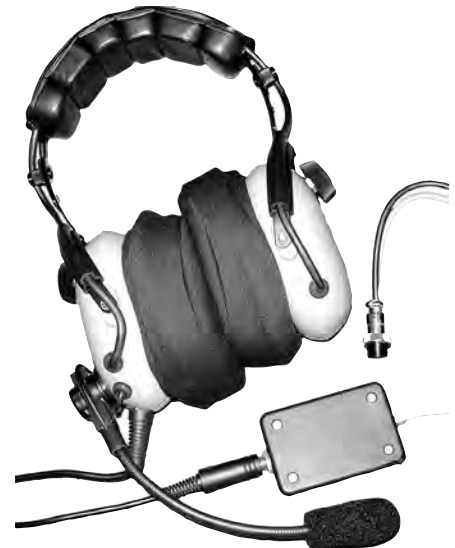
Fig 24.56 — A completed KØIZ headset/ adapter. The black box contains the adapter circuit for the aviation headset.
