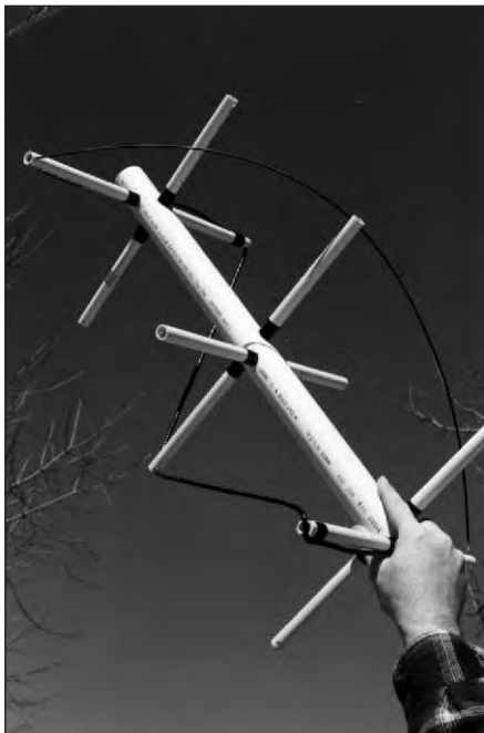
Fig 55 — The antenna with two of the four legs (filars) of one loop attached.
