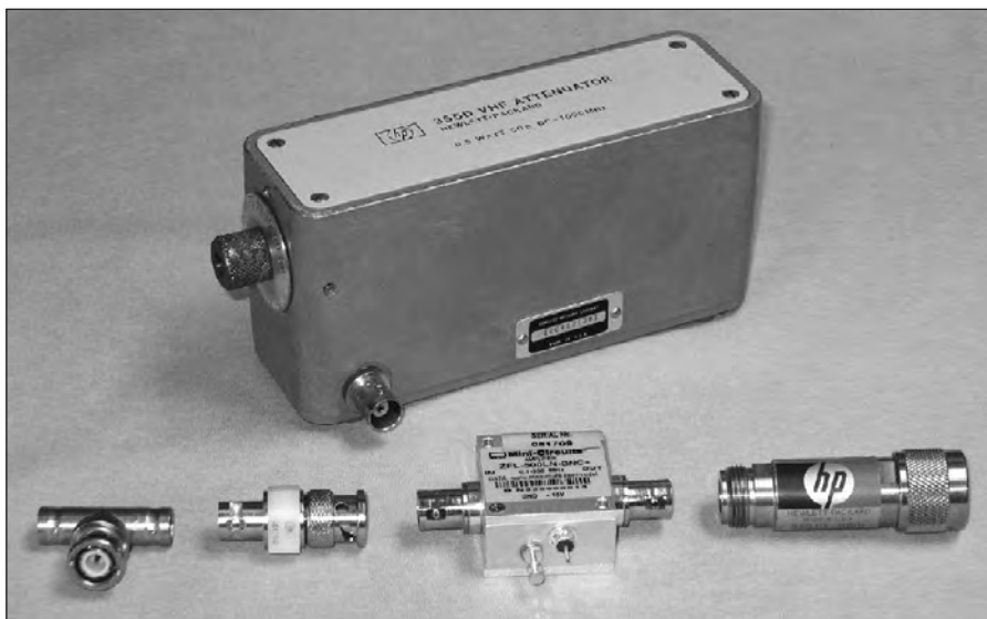
Fig 25.40 — Various RF test accessories. At the rear is a 10 dB step attenuator with a 0-120 dB range. In the foreground from left to right are a BNC "T" connector, a 50- \Omega feed-through termination, a 0.1-500 MHz low-noise amplifier, and a 10-dB fixed attenuator.
