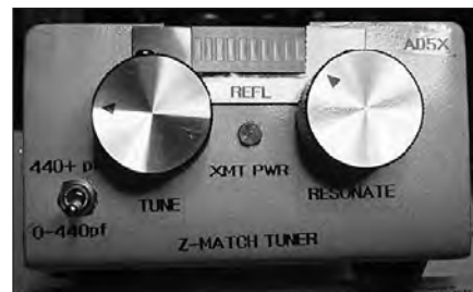
Fig 24.6 — The bar graph display of reflected power makes tuning easier and more intuitive.
