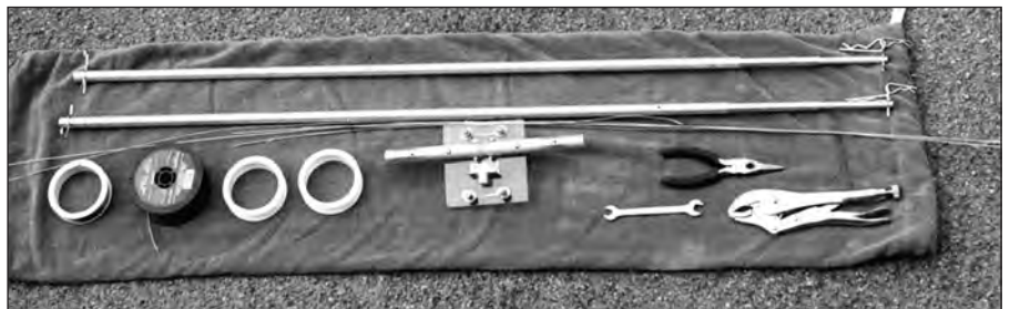
Fig 21.31 — The entire inverted-U antenna parts collection in semi-nested form, with its carrying bag. The tools stored with the antenna include a wrench to tighten the U-bolts for the mast-to-plate mount and a pair of pliers to help remove end wires from the tubing.
