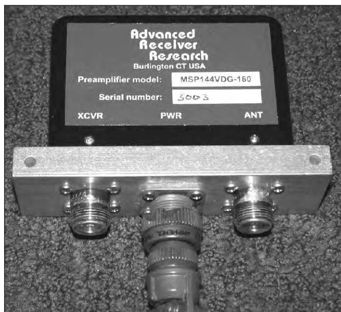
Fig 31 — This receive preamplifier by Advanced Receiver Research gives signals a substantial boost before they travel down the coaxial cable to your radio.
