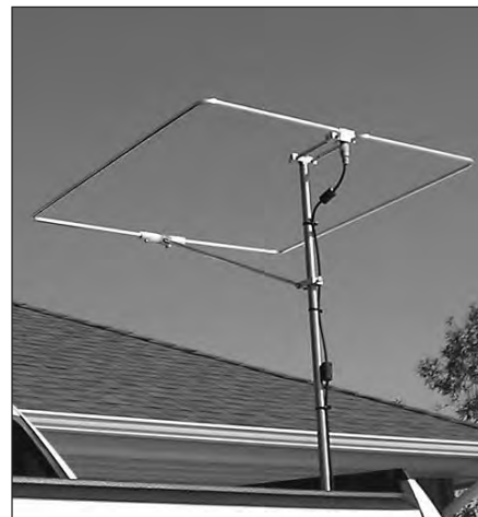
Fig 21.94 — The squalo (square halo) is a popular horizontally polarized VHF/UHF mobile antenna. The antenna shown here is made by M 2 Antenna Systems ( www.m2inc.com ).
