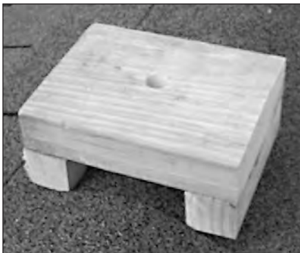
Fig 21.57 — At K8CH, the HVD base insulator sits in this saddle-shaped wooden fixture. This was photo was taken before the fixture was painted — a necessary step to protect against the weather.
