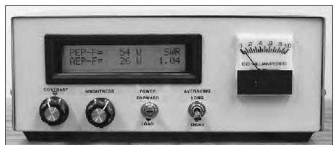
Fig 25.87 — Front panel of power meter. The LCD shows the peak envelope power (PEP), the average envelope power (AEP) and the SWR. The two knobs control the contrast and back lighting of the LCD. One toggle switch determines whether forward or load powers are displayed. A second switch sets the averaging time for the AEP calculation. The meter displays SWR and is used for tuning purposes.
