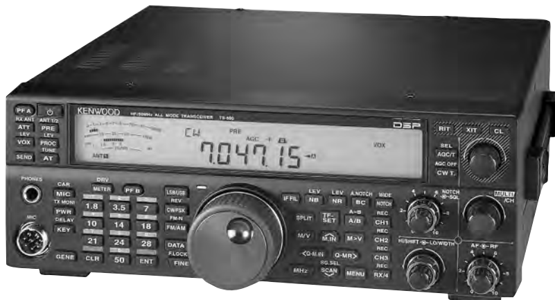
Fig 11 — The Kenwood TS-590S offers a high performance receiver on the primary HF amateur bands and many digital features.
