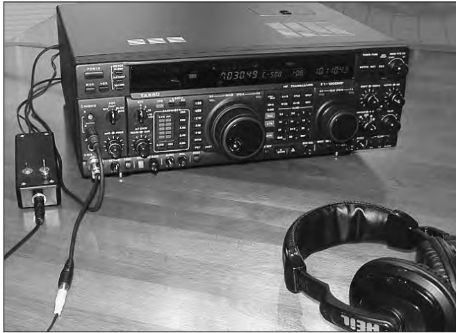
Fig 24.62 — The AIE takes up little desk space. It plugs inline between the transceiver and headphones and requires 13.6 V dc. In the author's shack, the unit is powered from a transceiver accessory jack and is always switched on.
