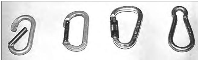
Fig 28.14 — (A) Oval mountain climbing type carabiners are ideal for tower workloads and attachments. The gates are spring loaded — the open gate is shown for illustration. (B) An open aluminum oval carabiner; a closed oval carabiner; an aluminum locking carabiner; a steel snaplink. (C) A heavy duty nylon sling on the left for big jobs and a lighter-duty loop sling on the right for everything else. (K7LXC photos)
