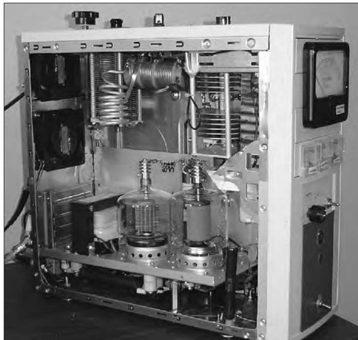
Fig 1.11 — Some hams enjoy building their own equipment, and many are quite good at repurposing or recycling outdated technology. Richard Calhoun, W6DZT, built this power amplifier in a discarded personal computer enclosure, bought through an online auction site for a few dollars. [Richard Calhoun, W6DZT, photo]
