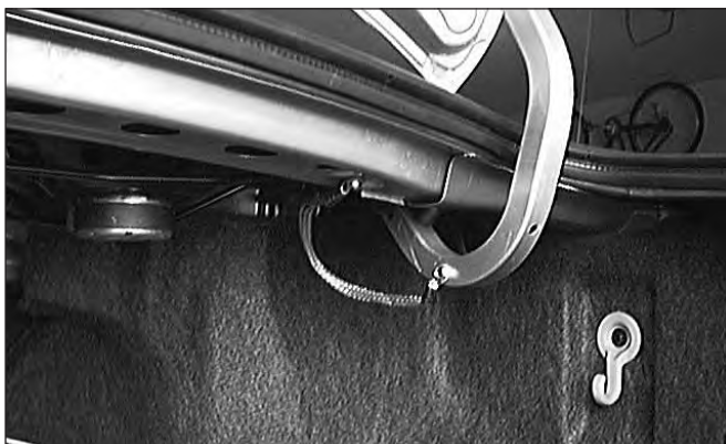
Fig 29.23 — Bonding vehicles parts — in this case, the trunk lid to the main body — can help reduce interference.
