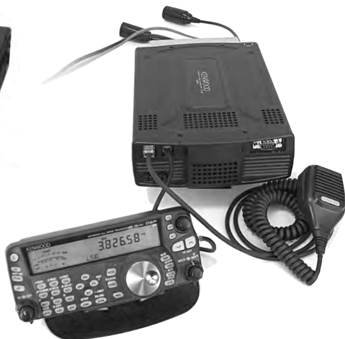
Fig 7 — Kenwood TS-480HX, the only transceiver in this category with a 200 W transmitter. The TS-480SAT looks similar, but offers 100 W output and an internal antenna tuner.
