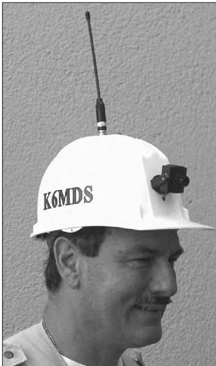
Fig 33 — Michael Saculla, K6MDS, built an ATV Hat Cam — www.hamtv.com/hatcam.html — using a CMOS color camera along with a Videolynx 70 cm transmitter for public service applications.
