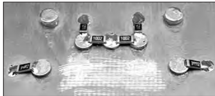
Fig 23.7D — SMT resistors soldered to base board of the Audio Amp in the beginning stages of assembly.
