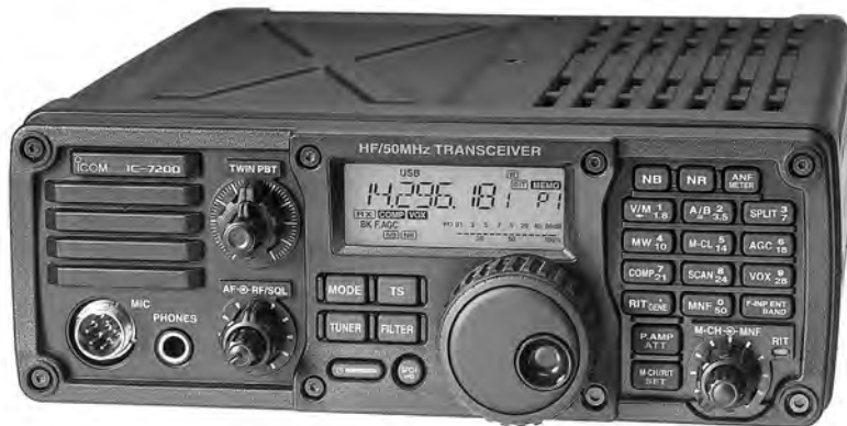
Fig 5 — The ICOM IC-7200 desktop HF and 6 meter transceiver — similar in size to the IC-718, but with an outdoor focus.
