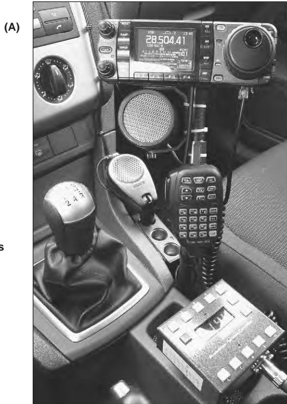
Fig 29.18 — At A, the transceiver control head is attached to one of many available mounts designed for this purpose. Mounts are typically highly adjustable, allowing the control head or radio to be positioned close to the operator. An antenna controller is mounted below the microphone. At B, HF and VHF transceiver control heads and the microphone are all mounted to the dashboard, within easy reach.
