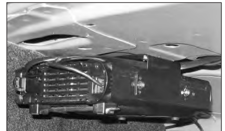
Fig 29.19 — The main body of the radio may be mounted in the vehicle's trunk or other out-of-the-way spot. Allow for plenty of ventilation.
