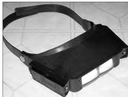
Fig 23.6 — A magnifying visor is great for close-up work on a circuit board. These headsets are often available for less than $10 at hamfests and some even come with superbright LEDs mounted on the side to illuminate the components being soldered.
