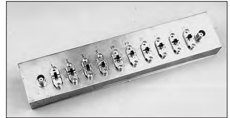
Fig 25.75 — The completed step attenuator in the enclosure of brass sheet. The BNC connectors may be mounted on the front panel at the end of the switches or on the end panels.
