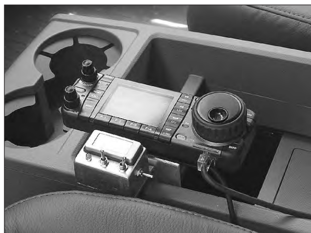
Fig 29.17 — In this mobile installation, the transceiver control head is mounted in the center console, next to a box with switches for adjusting the antenna.
