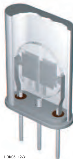
Fig 11.51 — A dual monolithic crystal filter has two sets of electrodes acoustically coupled to provide a two-pole response in a single crystal unit. The center lead is connected to the case and grounded in normal operation.
