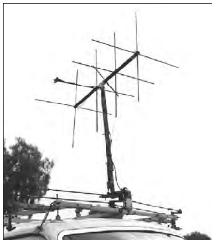
Fig 21.119 — The mobile RDF installation of WB6ADC features a thin wire quad that can be switched between vertical and horizontal polarization.
