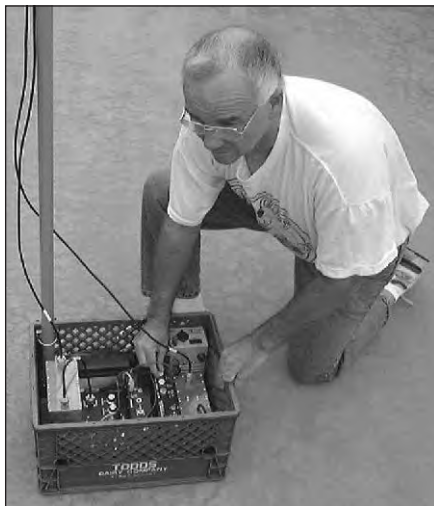
Fig 26 — At A, Tom O'Hara, W6ORG, adjusts a portable ATV repeater for public service work that can be built in a milk crate. The block diagram is similar to Fig 14 but without the VSB filters. The transmitter is a PC Electronics RTX23-3 on 1253.25 MHz, the receiver is on 426.25 MHz, and small beams or omni antennas are used. For more details on construction, visit www.hamtv.com/info.html#portrpt . At B, the repeater is flown to a hilltop and quickly set up. Sharon Kelly, KF6OQO, is adjusting the antenna. At C, the video of a fire can be seen at an EOC on the other side of the hill while Gary Heston, W6KVC, talks back to the incident site ATV operator on 2 meters.
