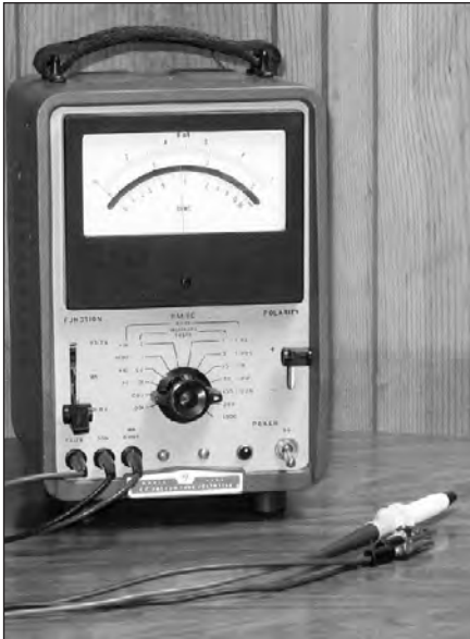
Fig 25.3 — This classic Hewlett-Packard HP412A vacuum-tube voltmeter (VTVM) has specifications that put many modern solid-state multimeters to shame.
