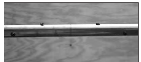
Fig 21.53 — Element splice uses a 1 foot length of 0.75 inch tubing inserted into the 0.875 inch sections to join them together. Self-tapping sheet-metal screws are used in this photo, but aluminum pop rivets or machine screws with washers and nuts can be used.
