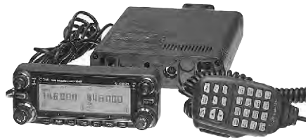
Fig 36 — The ICOM IC-2820 FM transceiver can receive and transmit on 2 m and 70 cm independently. With a dual-band FM rig like this, you can communicate through the FM repeater satellites, even while mobile.
