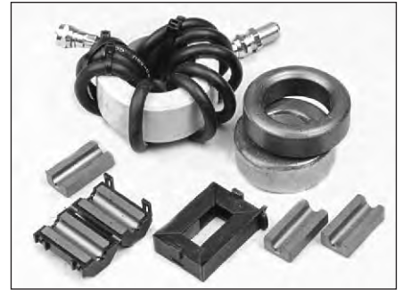
Fig 27.17 — A common-mode RF choke wound on a toroid core is shown at top left. Several styles of ferrite cores for common-mode chokes are also shown.
