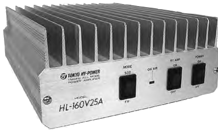
Fig 42 — A 150 W 2 meter RF power amplifier by Tokyo Hy-Power.
