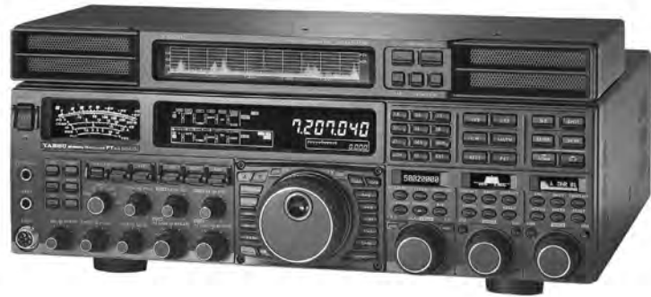
Fig 22 — The Yaesu FTDX5000MP is a top-performing 200 W transceiver, featuring a 300 Hz roofing filter and the companion SM-5000 station monitor.
