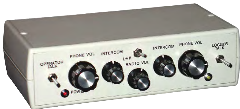
Fig 24.63 — Front view of the audio interface box. Operator controls are on the left and logger controls are on the right.
