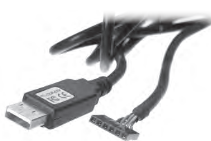
Fig 24.40 — The FTDI TTL-232R cable simplifies construction.
