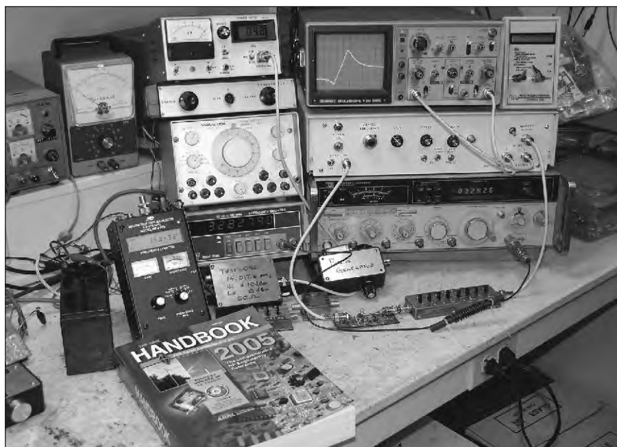
Fig 13.63 — The VE7CA work shop shows some of the home built and surplus test equipment used in the construction and evaluation of the HBR-2000.
