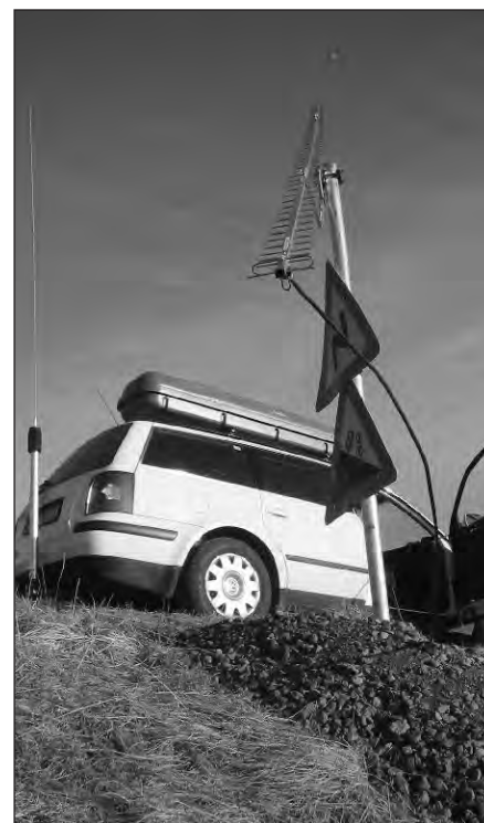
Fig 66 — TF/DL3OCH used a rural road sign to help him give contacts with Iceland to a number of EME operators on 1296 MHz. Bodo has activated many DXCC entities on 1296 MHz EME by using JT65, a single long Yagi and a 100 W solid state amplifier.
