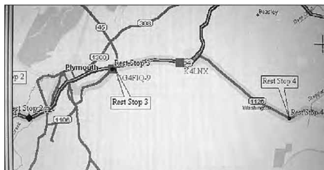
Fig 1.16 — APRS is a popular ham radio digital mode that allows tracking of mobile stations transmitting beacons via packet radio as they travel.
