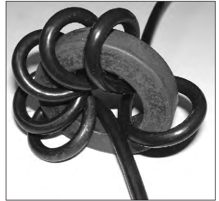
Fig 27.20 — To eliminate HF and VHF signals on the outside of a coaxial cable, use an 1- to 2-inch OD toroid core and wind as many turns of the cable on the core as practical.
