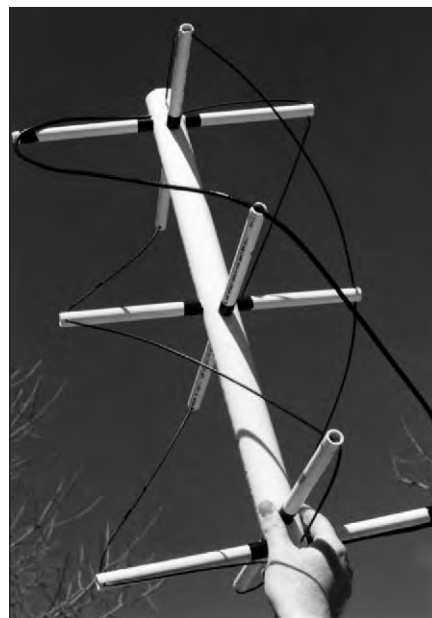
Fig 56 — This view shows the QHA with all four legs in place. The ends of the PVC cross arms that hold the coaxial leg are notched; the wire elements pass through holes drilled in the ends of their supporting cross arms.
