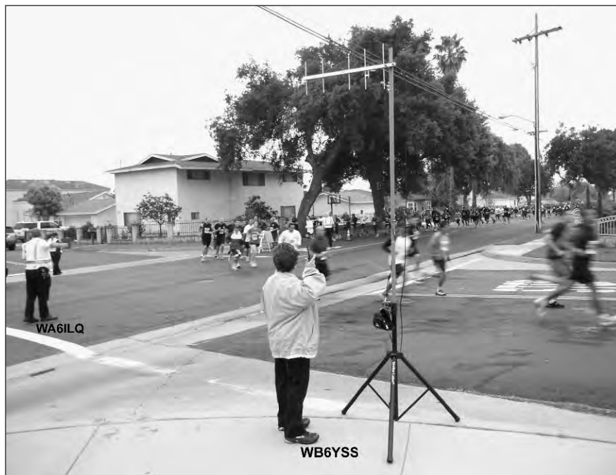
Fig 24 — A low power 50 mW battery operated portable 70 cm AM ATV transmitter is ideal for short range line of sight paths of up to 2 miles using 5 element beams. This setup can be used to show a critical intersection or condition of runners as an early warning to emergency response and aid station volunteers at races.
