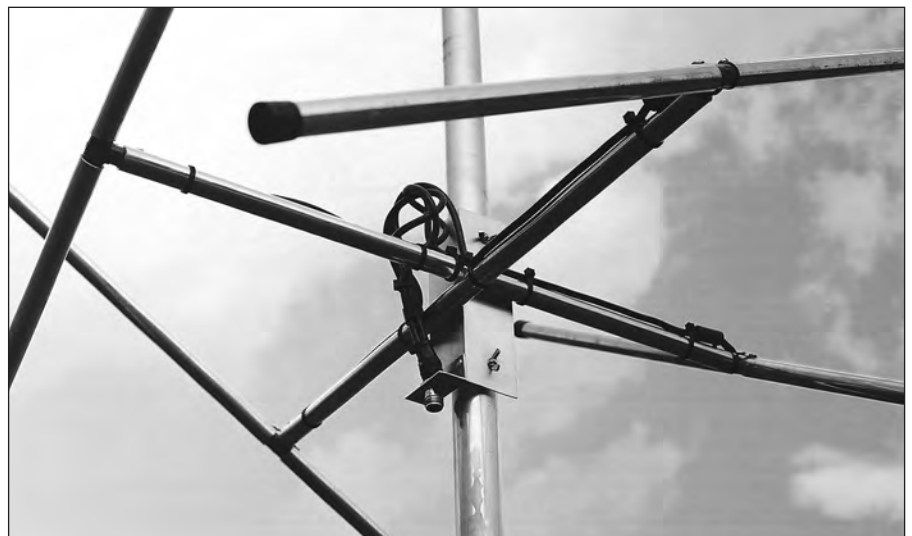
Fig 47 — View of cross booms mounted to mast.
