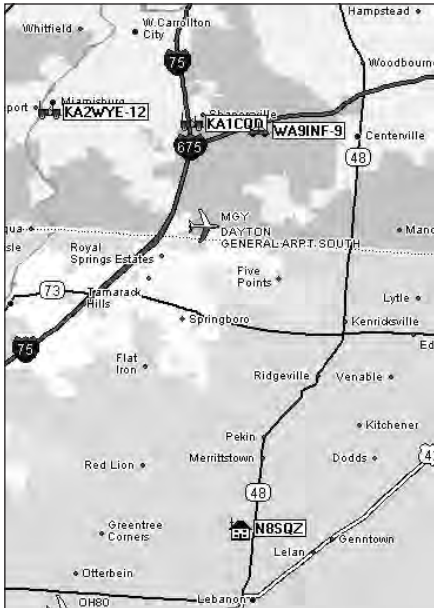
Fig 10 — A snapshot of APRS activity using UI-View software. Note the icons representing various mobile and fixed stations.
