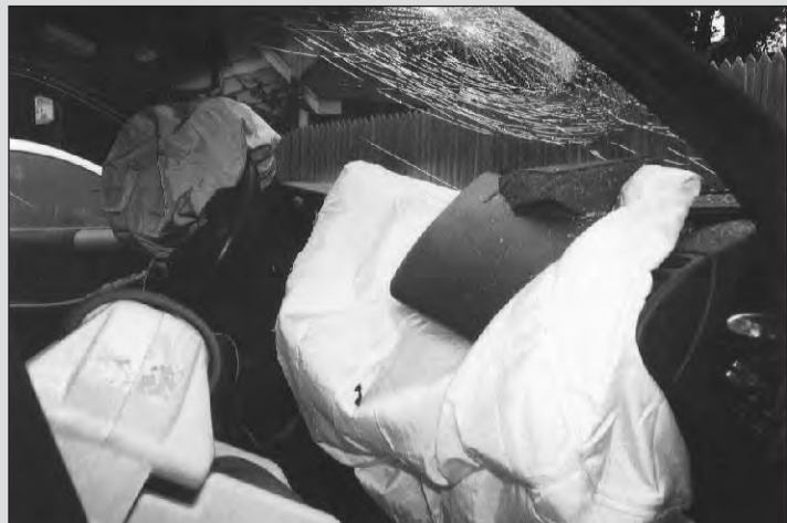
Fig 29.B — Airbag deployment following a minor collision caused significant disruption inside the passenger compartment.
