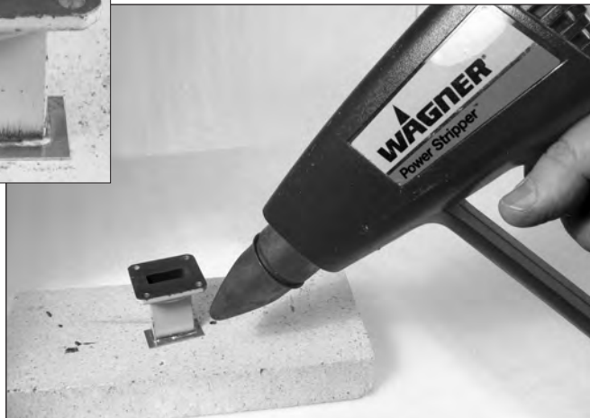
Fig 23.29 — Larger assemblies may be soldered with a heat gun. A torch is better for high-temperature brazing.
