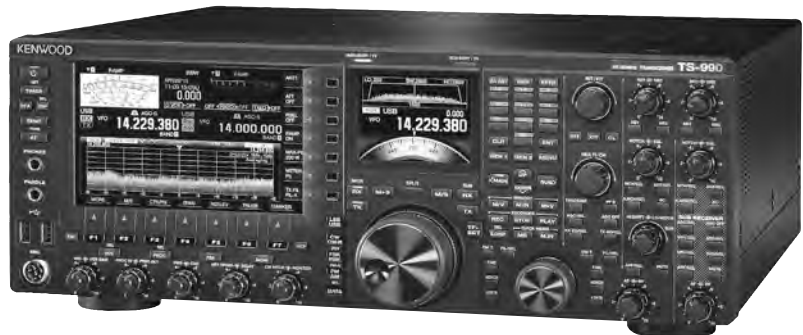
Fig 23 — The TS-990S is Kenwood's entry into the top-drawer category. It offers two receivers with high dynamic range, a 200 W transmitter and a host of interesting features.
