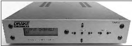
Fig 4 — The Drake DSE24 D-CATV 64-QAM modulator used for cable TV can be adapted for ATV with the addition of linear amplifiers. Maximum output is about -8 dBm which can drive high linearity MMIC, MOSFET and LDMOS amplifiers to usable power levels for ATV on the 70 cm and 33 cm bands. Transverters can be used for operation on higher frequency bands.
