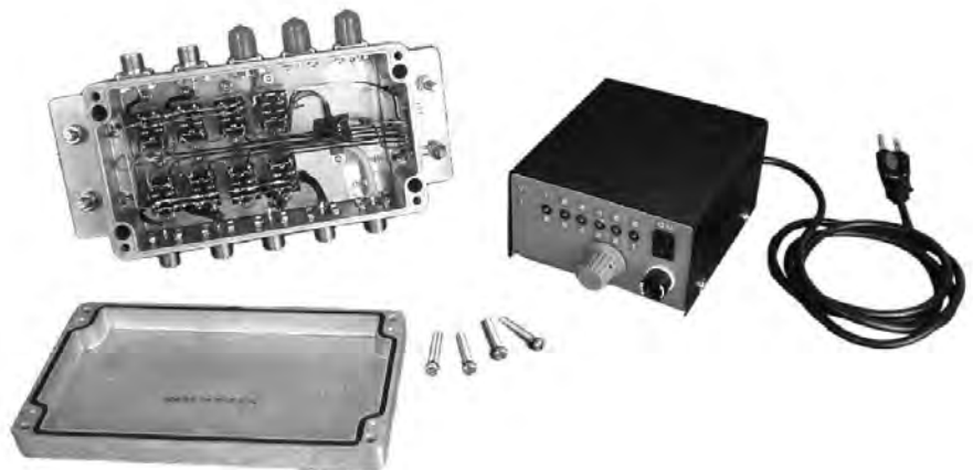
Fig 24.22 — Automatic antenna switch relay box (left) and control box (right).
