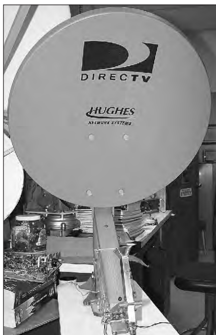
Fig 24 — This is a good example of an offset-fed dish. Note the feed source at the bottom edge of the photo, pointing into the center of the parabola. Also note that this is a DirectTV satellite TV antenna that has been “repurposed” for Amateur Radio satellites!
