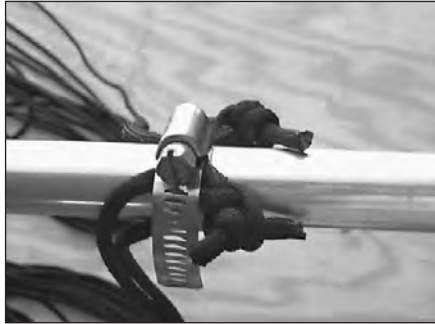
Fig 21.56 — Guys are made of Dacron line that is attached to the HVD by a stainless-steel worm-screw-type hose clamp. A self-tapping sheet-metal screw (not visible in the photo) prevents the clamp from sliding down the antenna.
