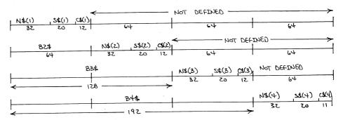
Figure 8.3 255-Byte Buffer Description by Four FIELD Statements
