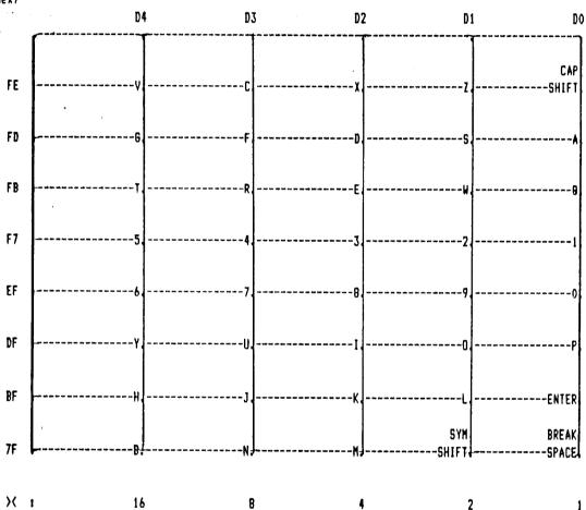
There are 4 main operations to test if a particular key has been pressed e.g. to check the "A" key:-
