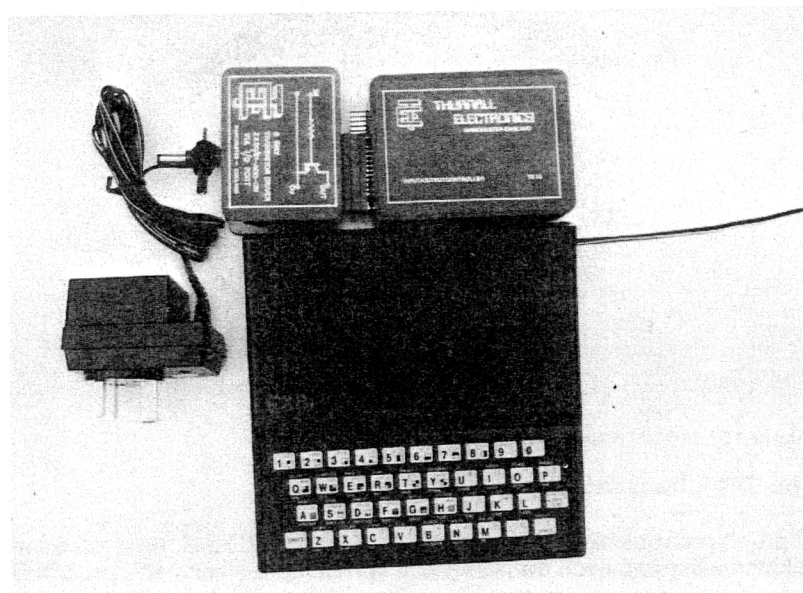
Figure 17a: ZX81, TE10 and TE15 and power supply, showing power supply inputs all connected
