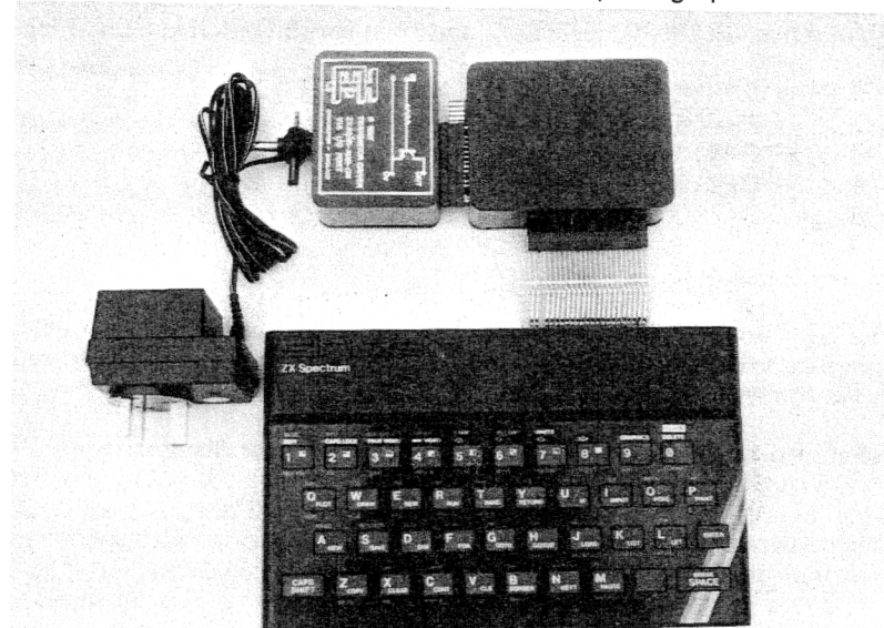
Figure 17b: Spectrum TE130 and TE15 and power supply, showing power supply inputs all connected.
