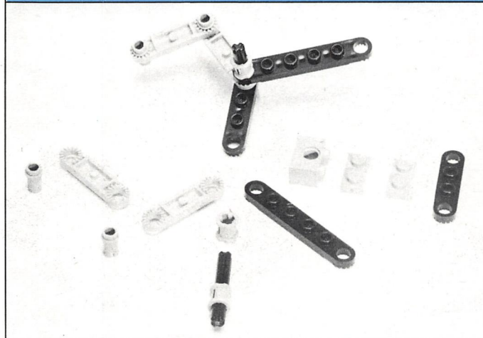
18 The fingers are made from steering links, which must all face in the directions shown here. One finger is shown made up, the other finger and the linkages as separate components.
