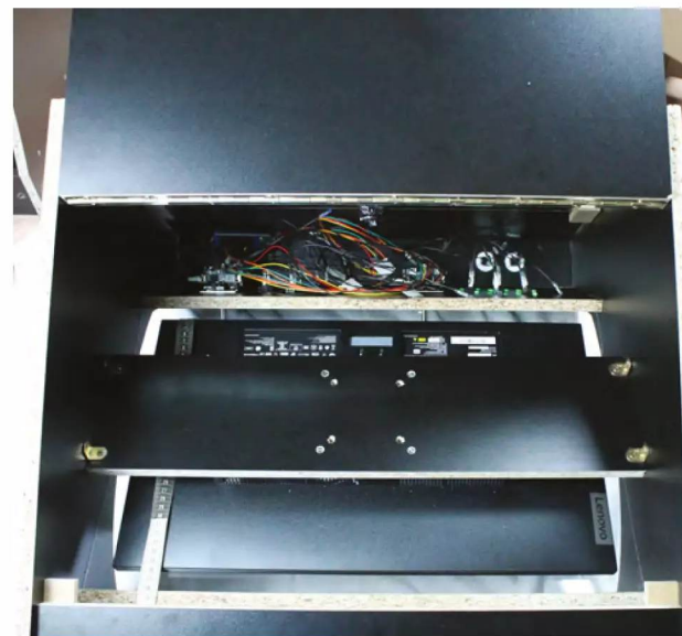
▲ To fit the VESA mount, place the cabinet face-down, then put the mounted monitor face-down on the front acrylic screen. Use a tape measure to help with positioning.
