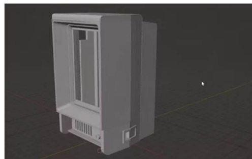
▶ Brendan designed the Vectrex Mini case in Blender and 3D-printed it
