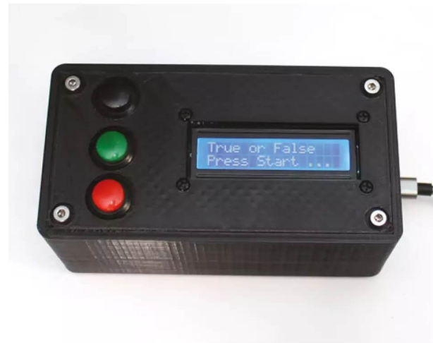
▲ Figure 7: The game can be placed inside an enclosure. If you don't have a 3D printer, you can use a generic case and cut appropriate holes
