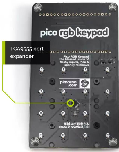
▲ Figure 4 The TCA9555 port expander is the small square integrated circuit mounted on the rear of the keypad PCB
