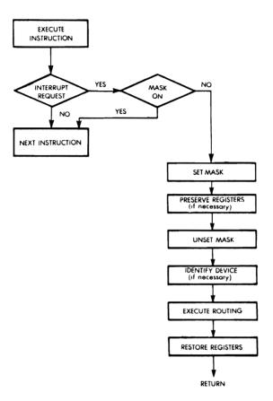
Fig. 6.34: Interrupt Logic
