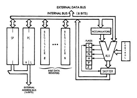
Fig. 2.2: "Standard" Microprocessor Architecture
