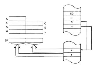
Timing: 6 M cycles; 20 T states; 10 usec @ 2 MHz
