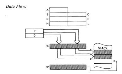
Timing: 3 M cycles; 11 T states; 5.5 usec @ 2 MHz Addressing Mode: Indirect. Byte Codes: p: 00 80 10 18 20 28 30 38 CF DF EF FF D7 E7 F7 Flags: (no effect). Example: 38H **RST** Before: After: PC [ PC 0038 441A SP 026B
