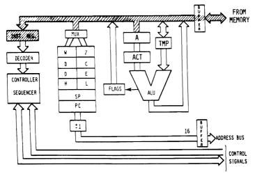
Fig. 2.19: The Instruction Arrives from the Memory into IR
