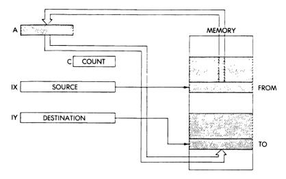
Fig. 5.7: Block Transfer: Initializing the Register
