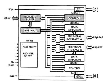
Fig. 7.2: Using a PIO-Load Control Register
