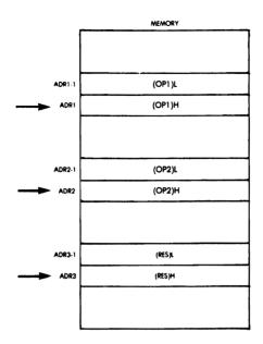
Fig. 3.7: Pointing to the High Byte
