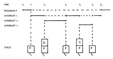
Fig. 6.33: Stack Contents During Multiple Interrupts
