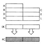
Timing: 2 M cycles; 8 T states; 4 usec @ 2 MHz
