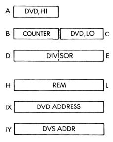
Fig. 3.34: Non-Restoring Division—The Registers
