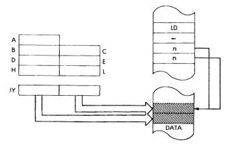
Timing: 6 M cycles; 20 T states; 10 usec @ 2 MHz
