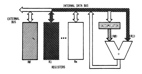
Fig. 2.10: Addition—Second Register R1 into ALU
