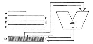
Timing: 2 M cycles; 10 T states; 5 usec @ 2 MHz
