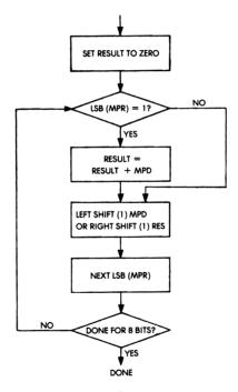
Fig. 3.12: The Basic Multiplication Algorithm—Flowchart
