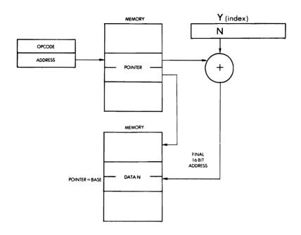
Fig. 5.3: Indirect Indexed Addressing (Post-Indexing)
