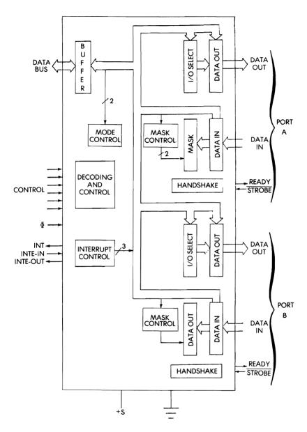
Fig. 7.7: Z80 PIO Block Diagram
