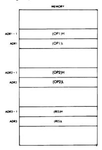
Fig. 3.5: 16-Bit Addition—The Operands
