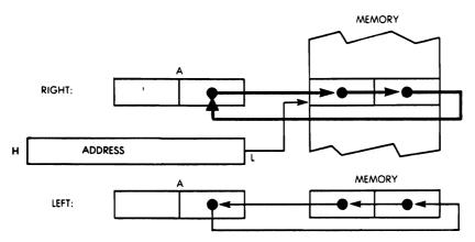
Fig. 4.13: Digit Rotate Instructions (Rotate Decimal)
