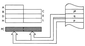
Timing: 3 M cycles; 10 T states; 5 usec @ 2 MHz
