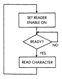
Fig. 6.20: Reading from a Paper-Tape Reader
