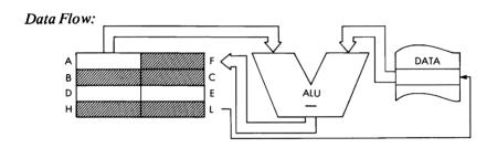
Timing: 4 M cycles; 16 T states: 8 usec @ 2 MHz
