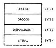
Fig. 5.5: Indexed Addressing Has 2-byte Opcode
