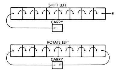
Fig. 4.1: Shift and Rotate
