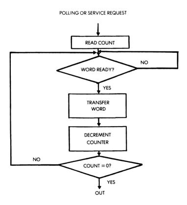
Fig. 6.5: Parallel Word Transfer: Flowchart
