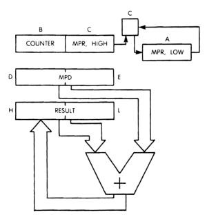
Fig. 3.27:  $16 \times 16$  Multiply—The Registers
