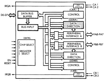
Fig. 7.3: Using a PIO-Load Data Direction
