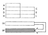
Timing: 2 M cycles; 10 T states; 5 usec @ 2 MHz
