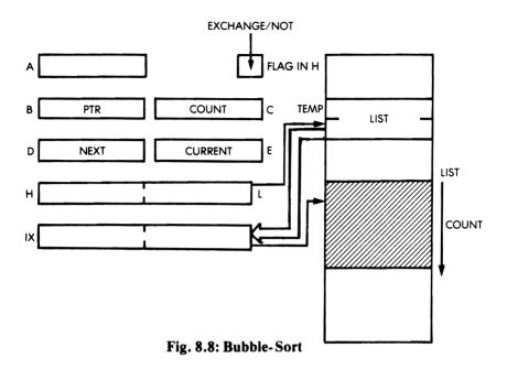
The register and memory assignments are shown on Figure 8.8, and the program is:
