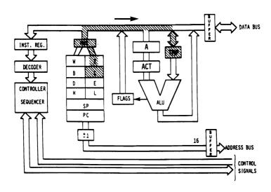
Fig. 2.21: The Contents of C Are Deposited into TMP
