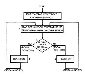
Fig. 1.1: A Flowchart for Keeping Room Temperature Constant
