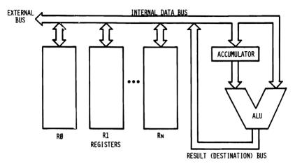
Fig. 2.8: Single-Bus Architecture
