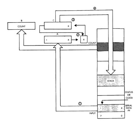
Fig. 6.7: Serial-to-Parallel: The Registers
