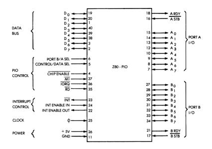
Fig. 7.6: Z80 PIO pinout
