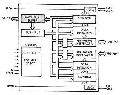
Fig. 7.4: Using a PIO-Read Status
