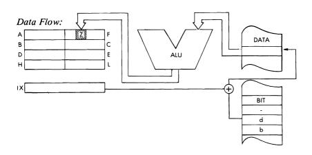
Timing: 5 M cycles; 20 T states: 10 usec @ 2 MHz
