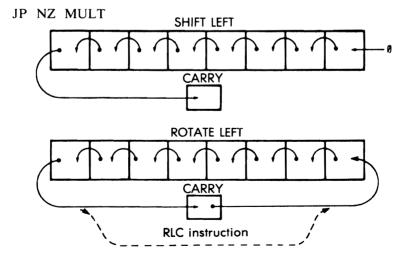
Fig. 3.17: Shift and Rotate
