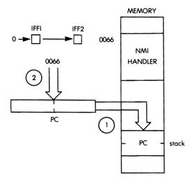
Fig. 6.25: NMI Forces Automatic Vectoring
