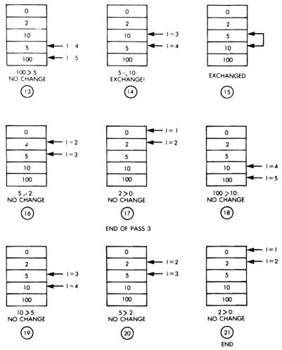
Fig. 8.6: Bubble-Sort Example: Phases 13 to 21
