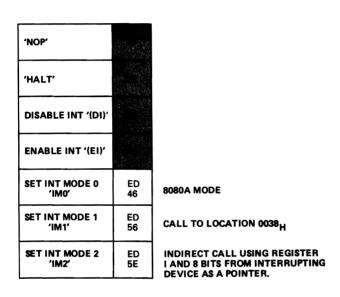
Fig. 4.22: Miscellaneous CPU Control
