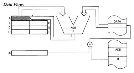
Timing: 5 M cycles; 19 T states: 9.5 usec @ 2 MHz
