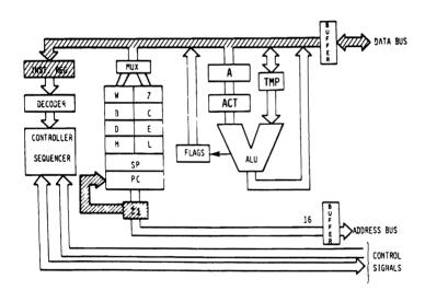
Fig 2.18: PC Is Incremented
