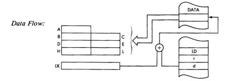
Timing: 5 M cycles; 19 T states; 9.5 usec @ 2 MHz
