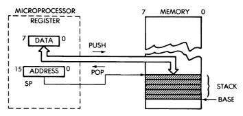
Fig. 2.5: The Two-Stack Manipulation Instructions
