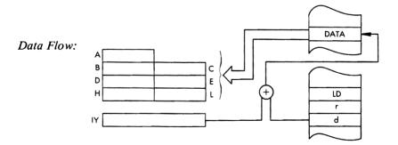
Timing: 5 M cycles, 19 T states; 9.5 usec @ 2 MHz
