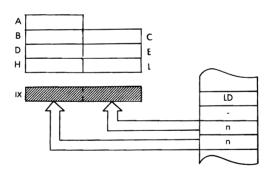
Timing: 4 M cycles; 14 T states; 7 usec @ 2 MHz
