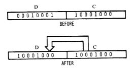
Fig. 2.20: Transferring C into D
