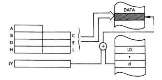
Timing: 5 M cycles; 19 T states; 9.5 usec @ 2 MHz
