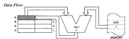
Timing: 2 M cycles; 7 T states: 3.5 usec @ 2 MHz
