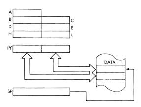
Timing: 6 M cycles; 23 T states; 11.5 usec @ 2 MHz
