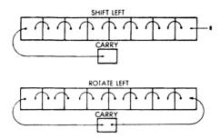
Fig. 4.9: Shift and Rotate
