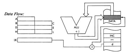
Timing: 6 M cycles; 23 T states; 11.5 usec @ 2 MHz
