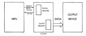
Fig. 6.8: Handshaking (Output)
