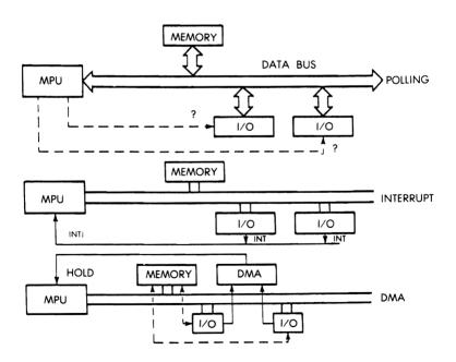
Fig. 6.18: Three Methods of I/O Control
