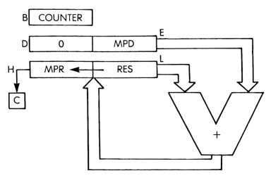
Fig. 3.25: Registers for Improved Multiply
