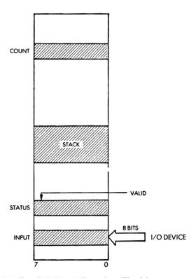
Fig. 6.4: Parallel Word Transfer-The Memory
