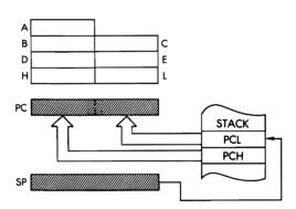
Timing: 3 M cycles; 10 T states; 5 usec @ 2 MHz
