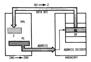
Fig. 2.32: Second Byte of Instruction Goes into Z
