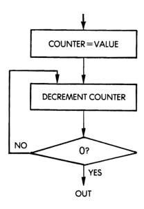
Fig. 6.3: Basic Delay Flowchart
