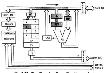
Fig. 2.23: Two Transfers Occur Simultaneously
