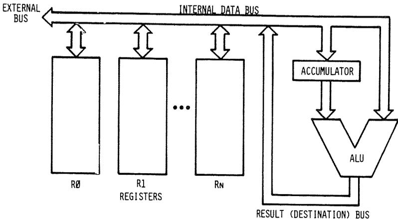
**Fig. 2.8: Single-Bus Architecture**
