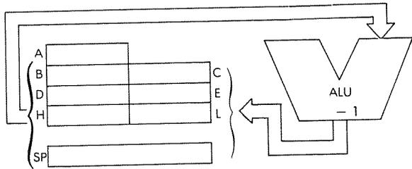
*Timing:*                              1 M cycle; 6 T states; 3 usec @ 2 MHz
