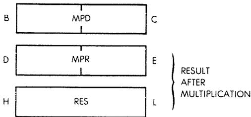
**Fig. 3.29: 16 × 16 Multiply with 32-Bit Result**
