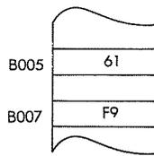
**LD (IX + d), n** Load indexed addressed memory location (IX + d) with immediate data n.
