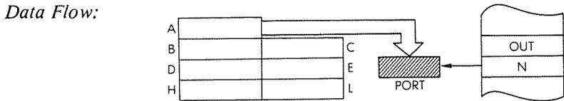
*Timing:*            3 M cycles, 11 T states; 5.5 usec @ 2 MHz
