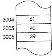
**PUSH qq** Push register pair onto stack.
