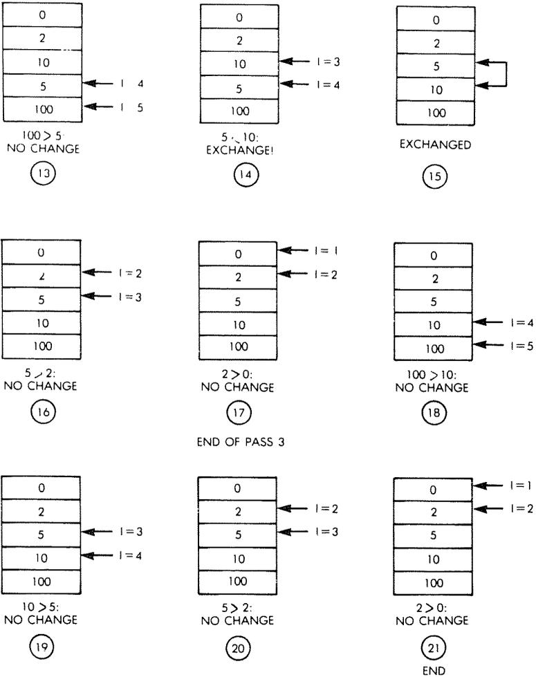
**Fig. 8.6: Bubble-Sort Example: Phases 13 to 21**
