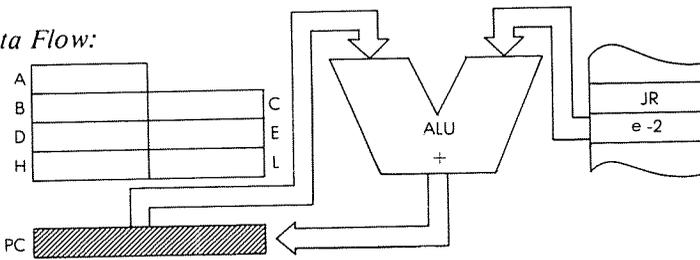
*Timing:* 3 M cycles; 12 T states; 6 usec @ 2 MHz
