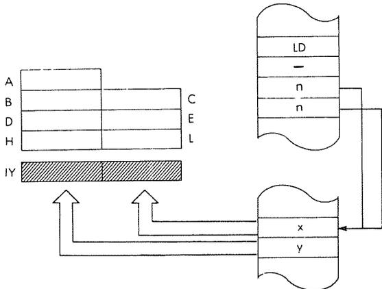
*Timing:* 6 M cycles; 20 T states; 10 usec @ 2 MHz
