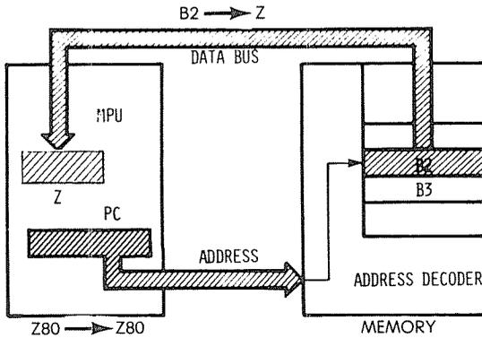
**Fig. 2.32: Second Byte of Instruction Goes into Z**
