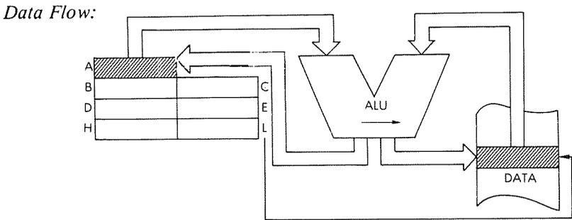
*Timing:* 5 M cycles; 18 T states; 9 usec @ 2 MHz
