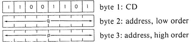
*Description:* The contents of the program counter are pushed onto the stack as described for the PUSH instructions. The contents of the memory location immediately following the opcode are then loaded into the low order half of the PC and the contents of the second memory location after the opcode are loaded in the high order half of the PC. The next instruction will be fetched from this new address.
