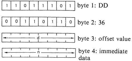
*Description:* The contents of the memory location immediately following the opcode are transferred into the memory location addressed by the contents of the index register plus the given offset value.
