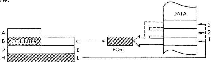
*Timing:*                              B = 0: 4 M cycles; 16 T states; 8 usec @ 2 MHz.
