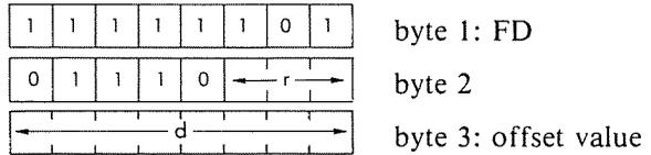
*Description:* The contents of the specified register are loaded into the memory location addressed by the contents of the index register plus the given offset value. r may be any one of:
