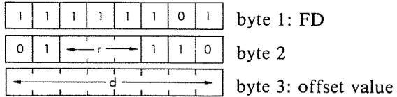
*Description:* The contents of the memory location addressed by the IY index register plus the given offset value, are loaded into the specified register. r may be any one of:
