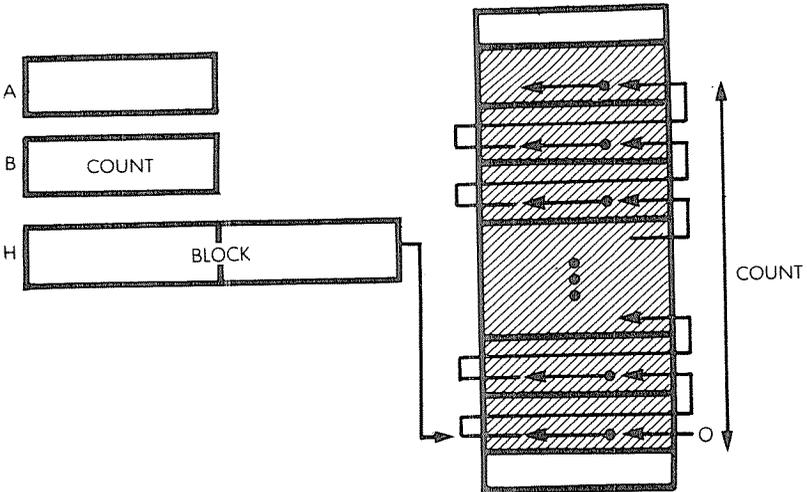
**Fig. 8.3: BCD Block Transfer - The Memory**
