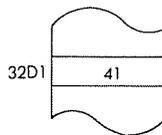
**LD A, (DE)** Load the accumulator from the memory location indirectly addressed by the DE register pair.
