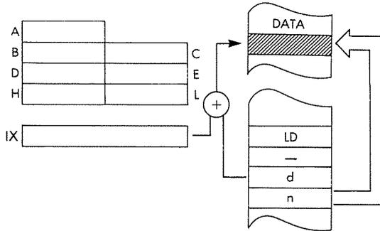
*Timing:* 5 M cycles; 19 T states; 9.5 usec @ 2 MHz
