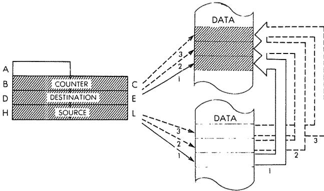
*Timing:*  $BC \neq 0$ : 5 M cycles; 21 T states; 10.5 usec @ 2 MHz.
