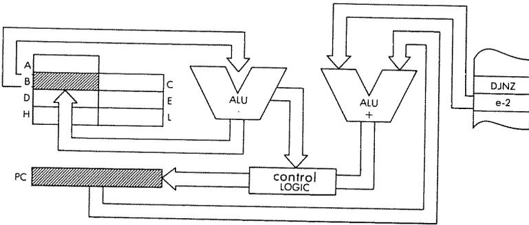
*Timing:*                               $B \neq 0$ : 3 M cycles; 13 T states; 6.5 usec @ 2 MHz.
