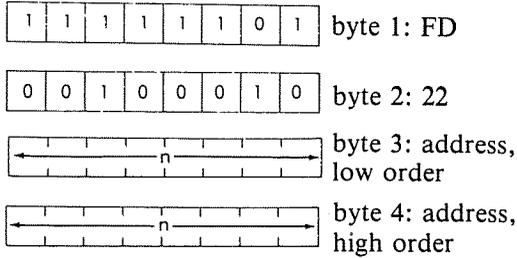
*Description:* The contents of the low order of the IY register are loaded into the memory location addressed by the contents of the memory location immediately following the opcode. The contents of the high order of the IY register are loaded into the memory location immediately following the one loaded from the low order. The low order of the nn address occurs immediately after the opcode.
