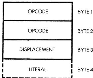
**Fig. 5.5: Indexed Addressing Has 2-byte Opcode**
