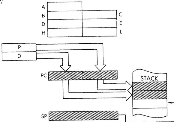
*Timing:* 3 M cycles; 11 T states; 5.5 usec @ 2 MHz
