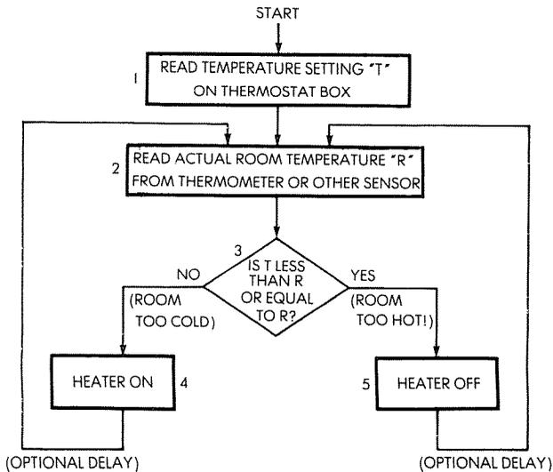
**Fig. 1.1: A Flowchart for Keeping Room Temperature Constant**
