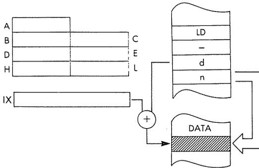
*Timing:* 5 M cycles; 19 T states; 9.5 usec @ 2 MHz
