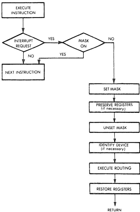
Fig. 6.34: Interrupt Logic
