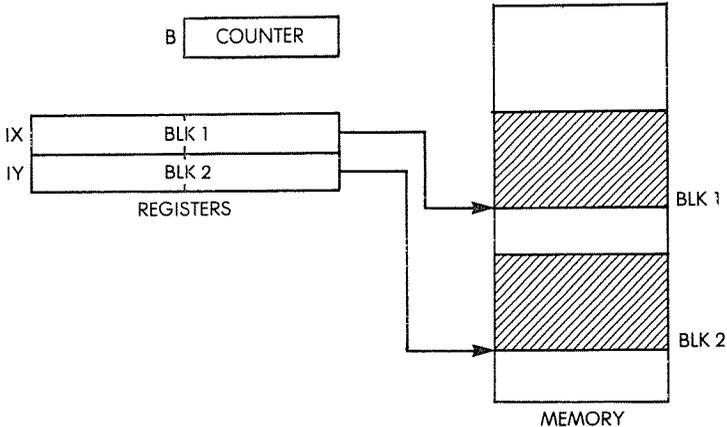
The memory layout is shown in Figure 5.9. The program is straightforward. The number of elements to be added is loaded into the counter register B, and the two index registers IX and IY are initialized to their values BLK1 and BLK2:
