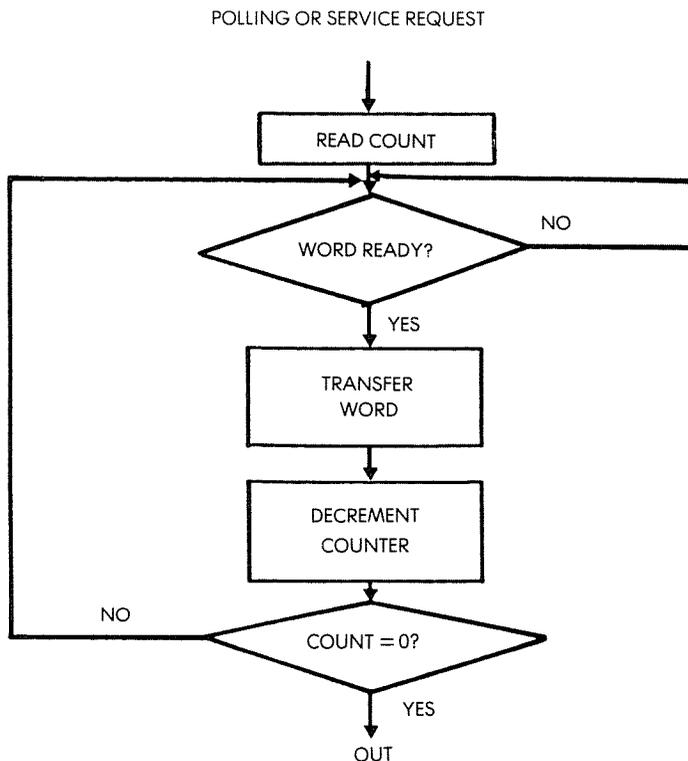
**Fig. 6.5: Parallel Word Transfer: Flowchart**
