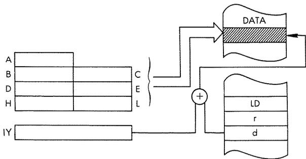
*Timing:* 5 M cycles; 19 T states; 9.5 usec @ 2 MHz
