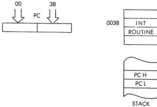
*Timing:* 2 M cycles; 8 T states; 4 usec @ 2 MHz
