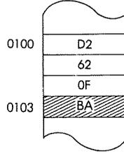
**LD (IX + d),r** Load indexed addressed memory location (IX + d) from register r.
