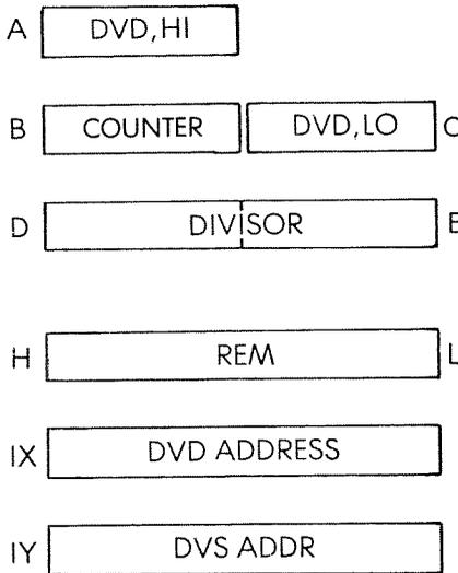
**Fig. 3.34: Non-Restoring Divisor—The Registers**
