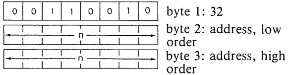
*Description:* The contents of the accumulator are loaded into the memory location addressed by the contents of the memory locations immediately following the opcode. The low byte of the address immediately follows the opcode.
