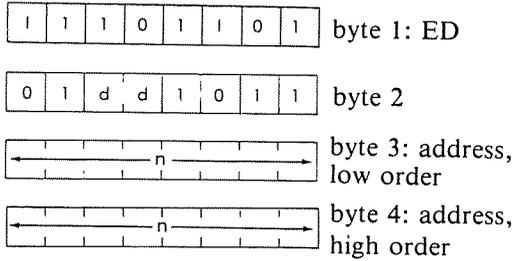
*Description:* The contents of the memory location addressed by the memory locations immediately following the opcode are loaded into the low order of the specified register pair. The contents of the memory location immediately following the one previously loaded are then loaded into the high order of the register pair. The low order byte of the nn address immediately follows the opcode. dd may be any one of:
