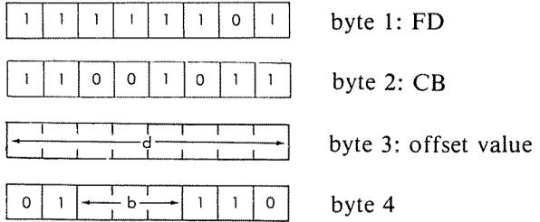
*Description:* The specified bit of the memory location addressed by the contents of the IY register plus the given offset value is tested and the Z flag is set according to the result. b may be any one of:
