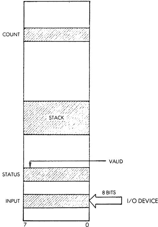
**Fig. 6.4: Parallel Word Transfer - The Memory**
