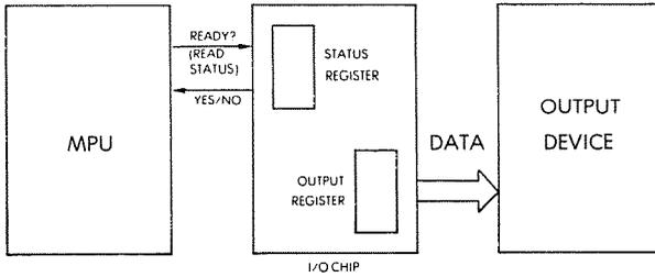
**Fig. 6.8: Handshaking (Output)**
