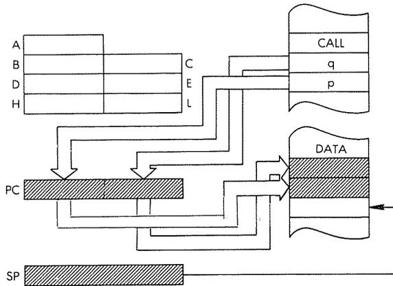
*Timing:* 5 M cycles; 17 T states: 8.5 usec @ 2 MHz
