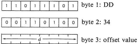
*Description:* The contents of the memory location addressed by the contents of the IX register plus the given offset value are incremented and stored back at that location.
