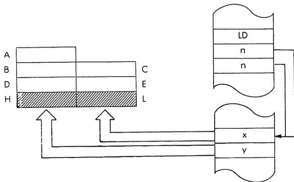
*Timing:* 5 M cycles, 16 T states; 8 usec @ 2 MHz
