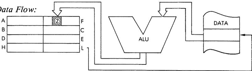
*Timing:* 3 M cycles; 12 T states; 6 usec @ 2 MHz
