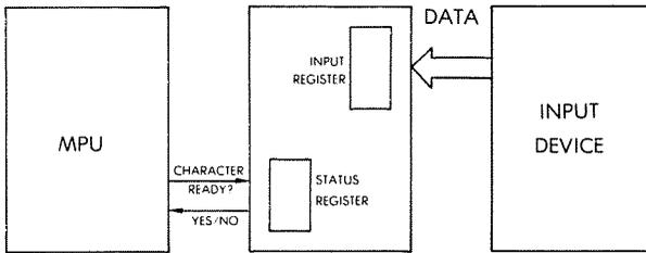
**Fig. 6.8a: Handshaking (Input)**
