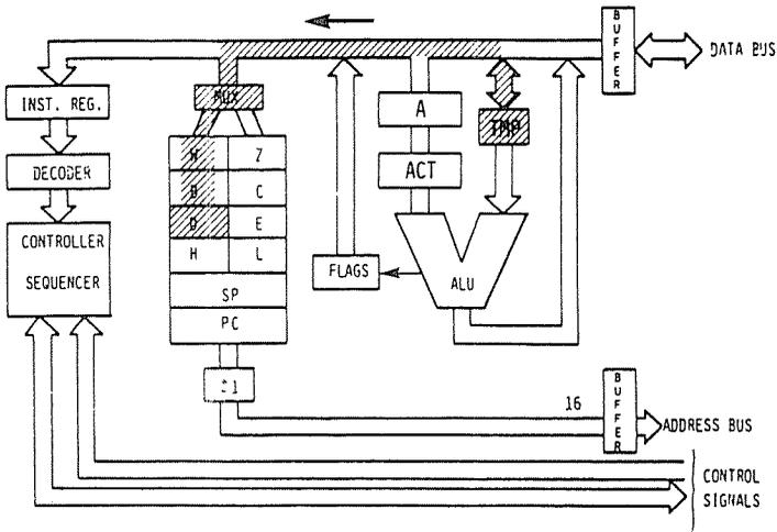
**Fig. 2.22: The Contents of TMP are Deposited into D**
