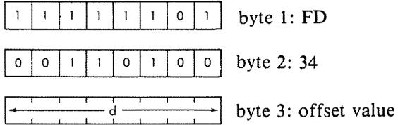
*Description:* The contents of the memory location addressed by the contents of the IY register plus the given offset value are incremented and stored back at that location.
