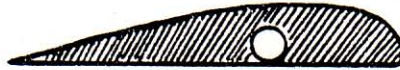
Figure 6.17 A cross section of the rotor paddle showing the embedded brass tubing.
