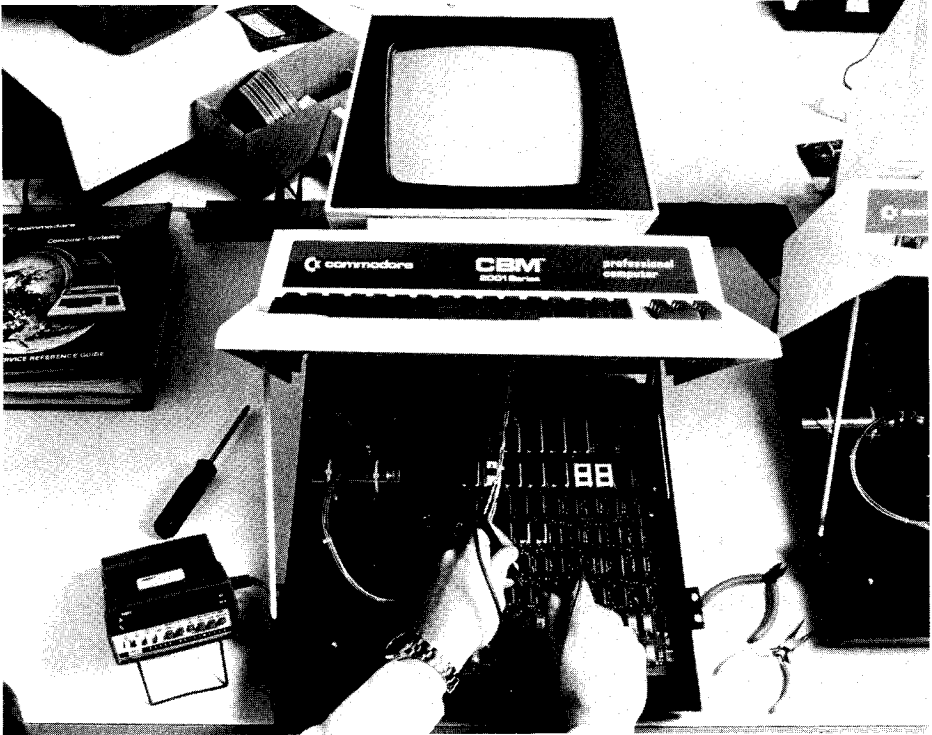
Figure 2-12. PET Internal View
