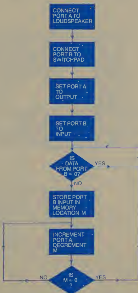
Figure 70: Flowchart for a simple electronic organ program
