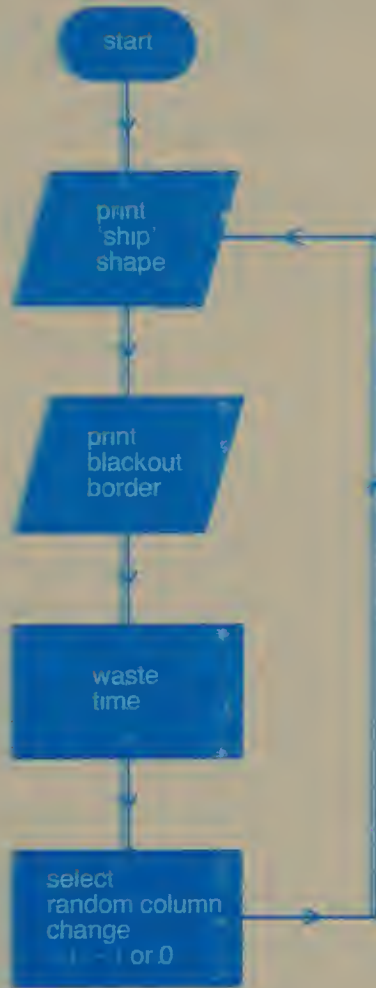
Figure 79: Flowchart for the 'Ship' program
