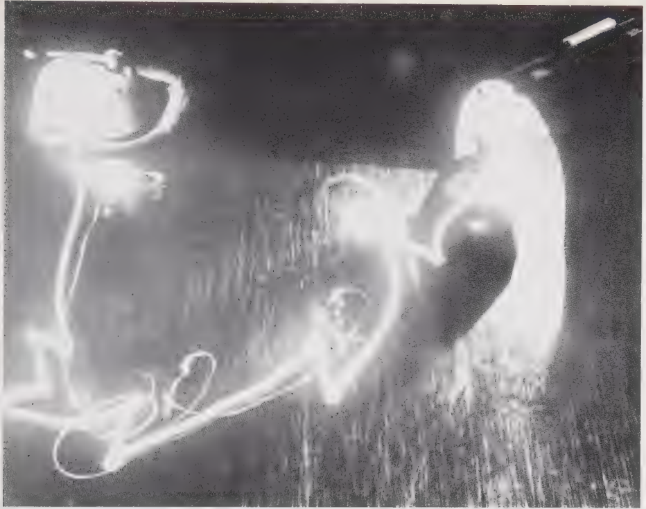
A time-lapse photograph of one of Grey Walter's tortoises making tracks towards the recharging station.
