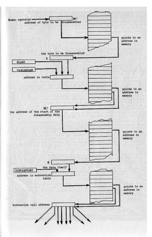
With these eight subroutines, which you will have to write yourself, you can disassemble every instruction. I will give you an example. Suppose CLASS is zero, and F is three. The first byte it has to interpret should be 00. This alters the value of HL' according to the quantity H, that is, bits 2, 1, and 0 of the byte being disassembled. Suppose now that H is one. HL' should now be pointing to the following sequence of data, listed here along with its meaning.
