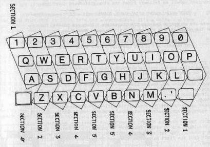
Now let's see what would happen if you pressed SHIFT S. Both bits zero and two would be reset giving, in binary, 11111010. In hex this is FA, so HL would return as FAFB - which is <u>different</u> to the value produced without shift. We can see the precise effect of SHIFT from this table:
