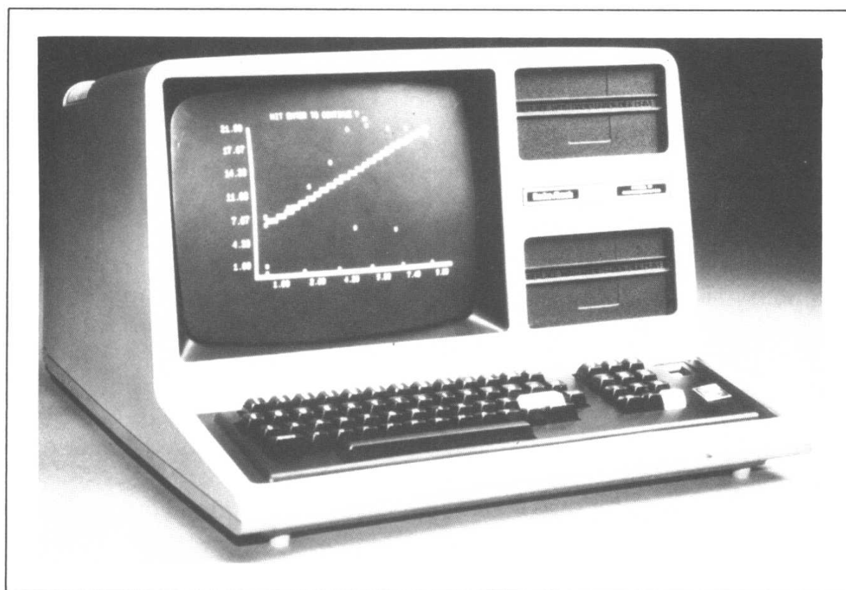
Figure 1.4 The Tandy TRS Model III with dual 5¼ inch floppy disk drive (178 kbytes each).
