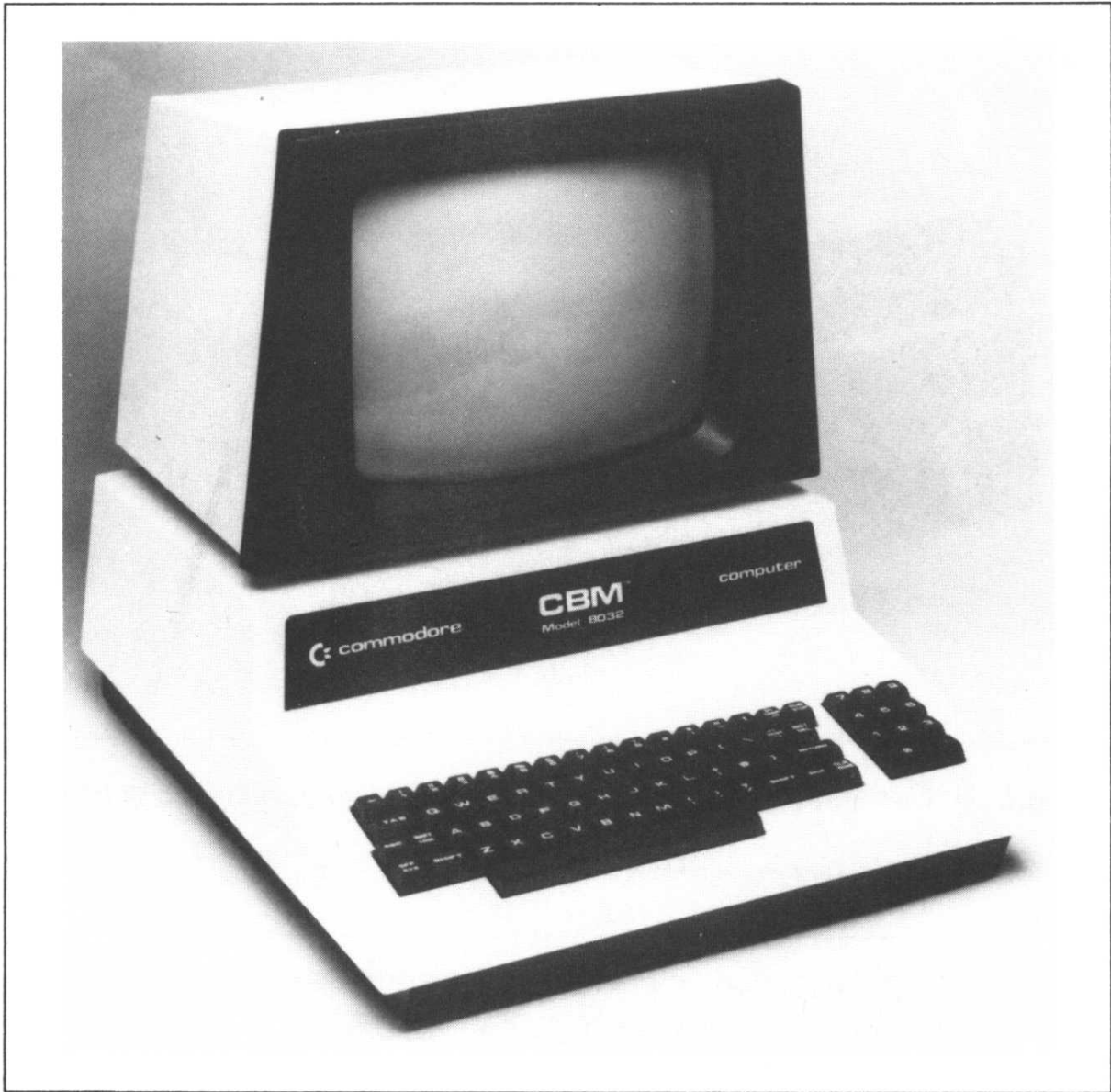
Figure 1.3a Commodore/Pet 8032 microcomputer, 32 kbytes of RAM and 80 column screen.
