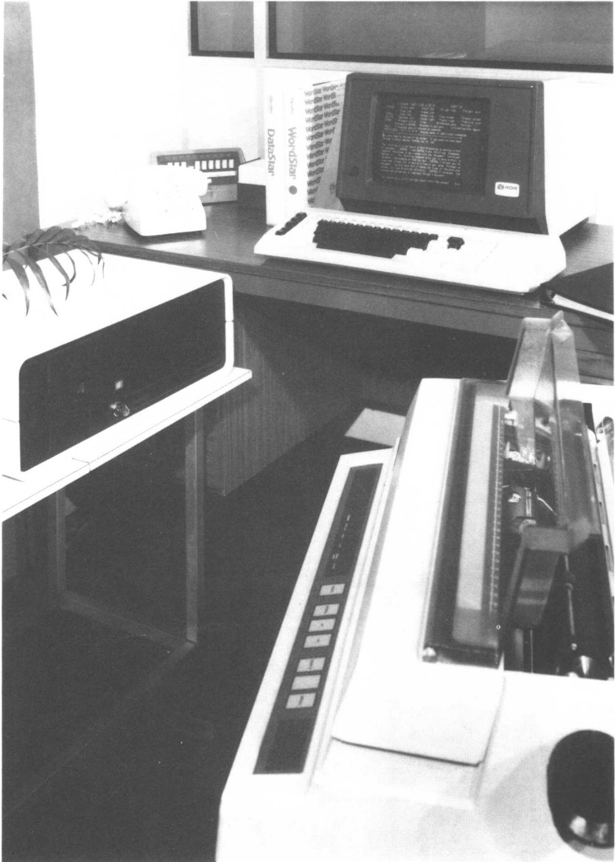
Figure 1.7 The British assembled Comart Communicator microcomputer with 5 1 / 4 inch floppy and 5 1 / 4 inch Winchester disk drives together with a Diablo daisy-wheel printer.
