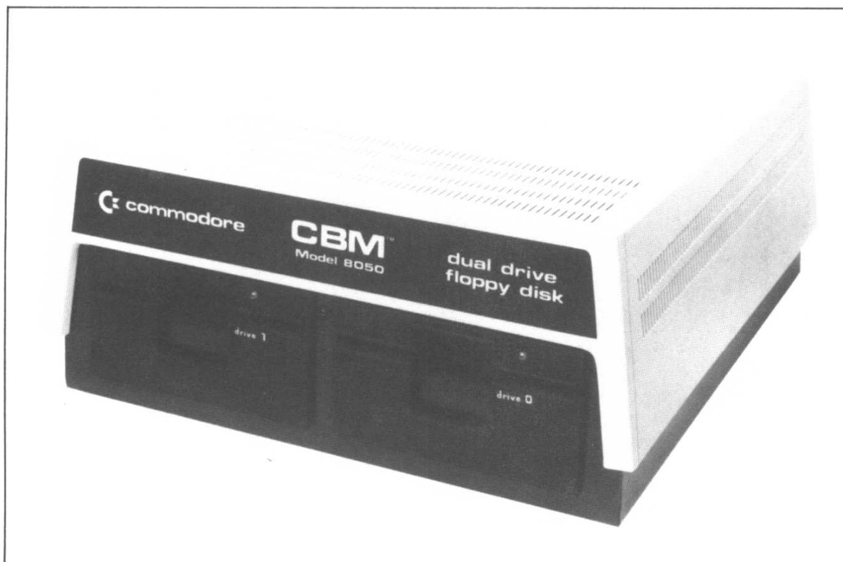
Figure 1.3b Commodore 8050 disk drive with 950 kbytes on two 5¼ inch disks.
