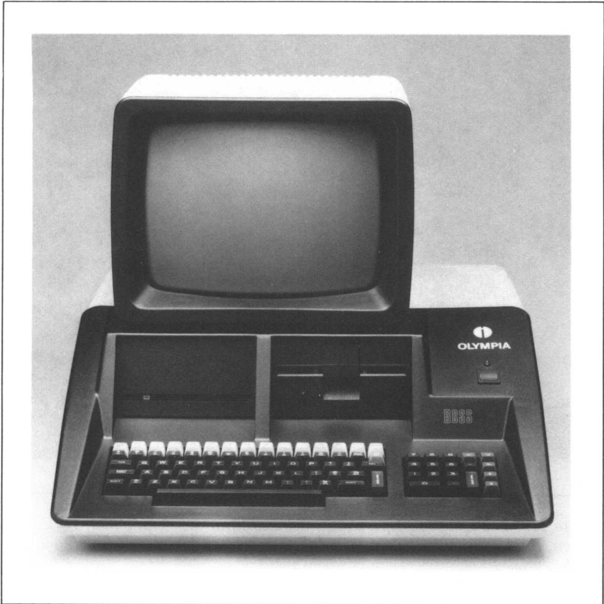
Figure 1.8 Olympia's Boss microcomputer with 5 1 / 4 inch floppy disk drive (600 kbytes) and 5 1 / 4 inch Winchester hard disk drive (5 Megabytes).
