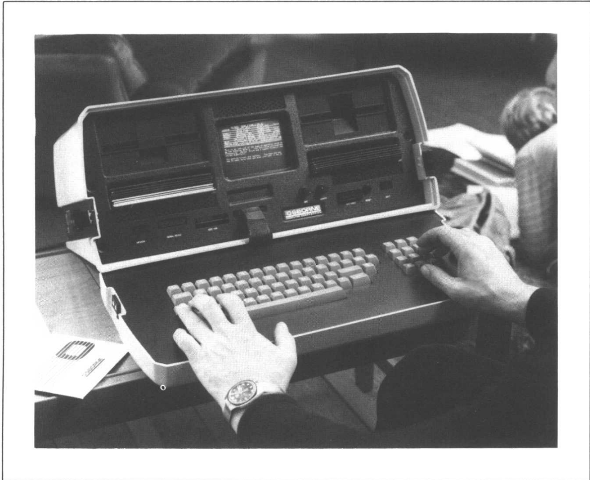
Figure 1.9 The Osborne 1 personal business computer with 5 inch VDU screen, dual floppy disk drives (100 kbytes each) and weighing only 24 lbs. Courtesy: Comart Ltd
