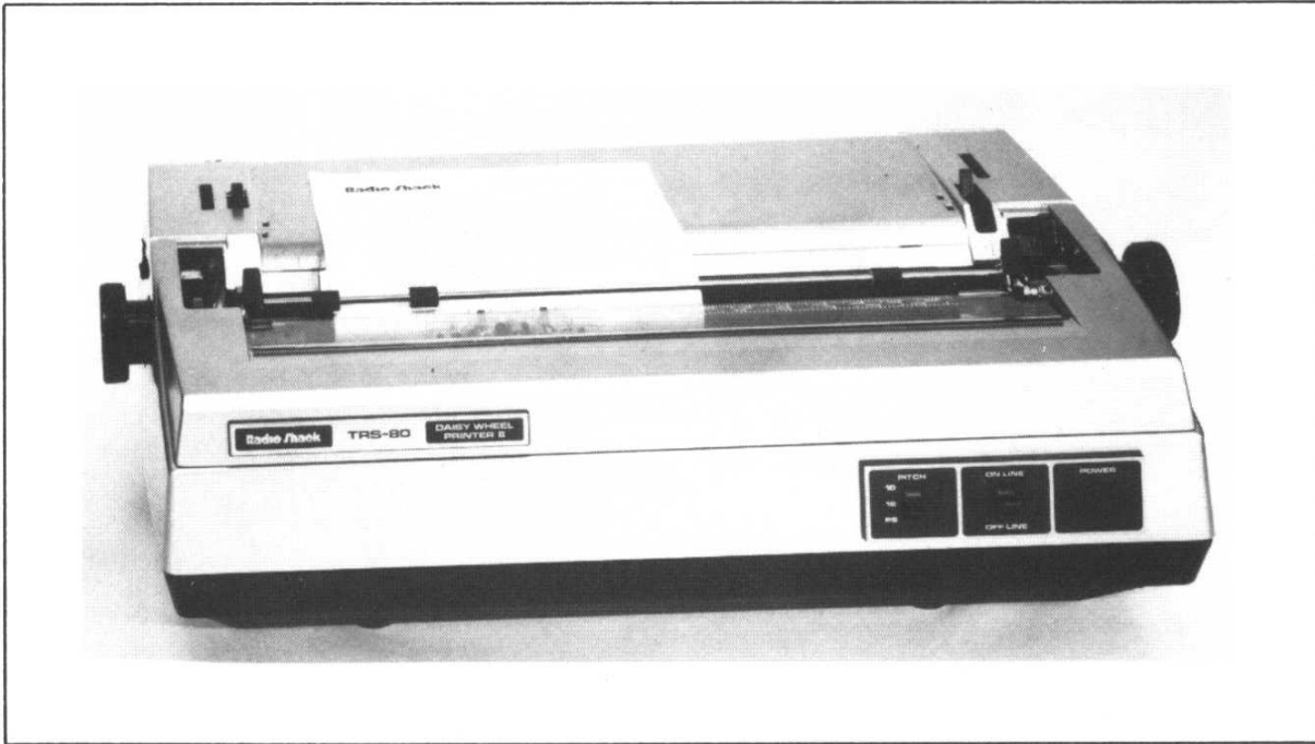
Figure 1.12 (above) Tandy TRS-80 Daisy-wheel II printer with a print speed of 43 cps and 136 characters per line. (left) Print daisy-wheel.
