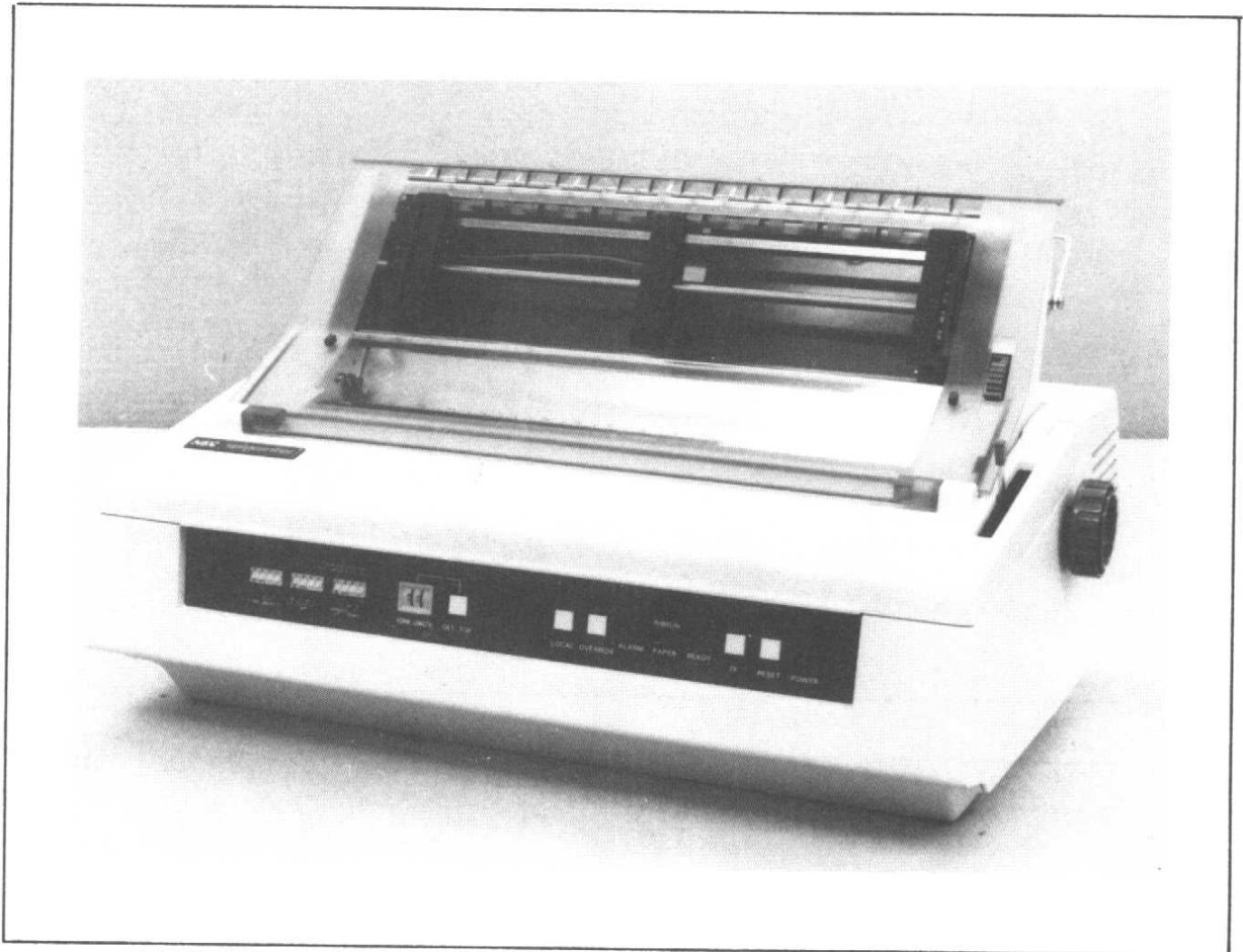
Figure 1.13 (above) NEC spin writer, high quality thimble printer (55 cps). (left) Print thimble.
