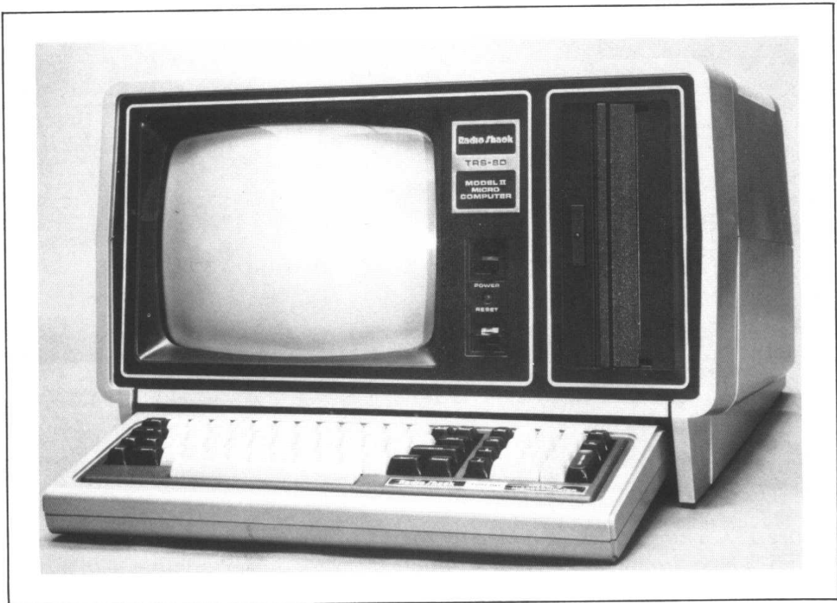
Figure 1.6 TRS-80 Model II microcomputer with up to 64 kbytes of RAM and 500 kbytes on a single large floppy disk. Courtesy: Tandy Corporation (Branch UK)
