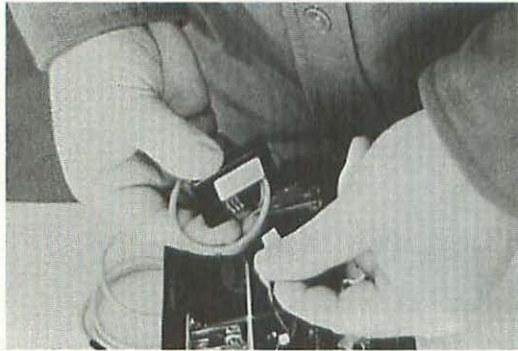
Figure 4-17 Plug the fan wires into the controller, then plug the controller wires into the PCB.
