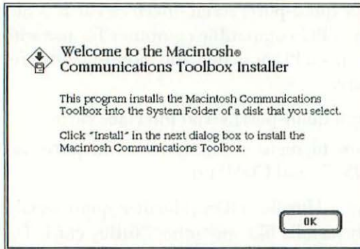
Figure 7-11 Use the Communications Toolbox Installer to add the CTB to Systems 6.0.4, 6.0.5, and 6.0.7.
