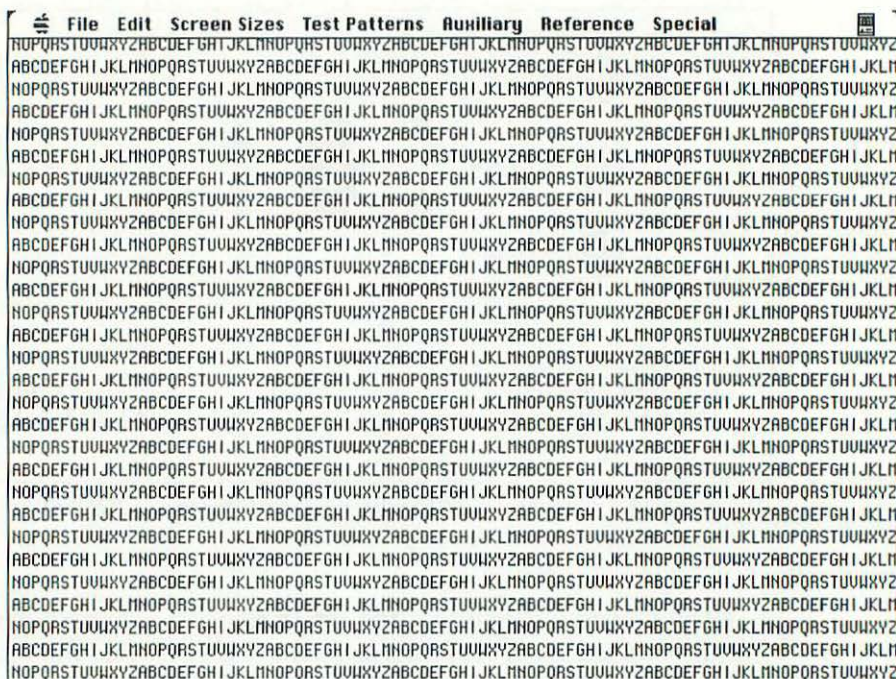
Figure 3-13 Holding down the Option key while choosing Focusing Text fills the display with 12-point Monaco text.
