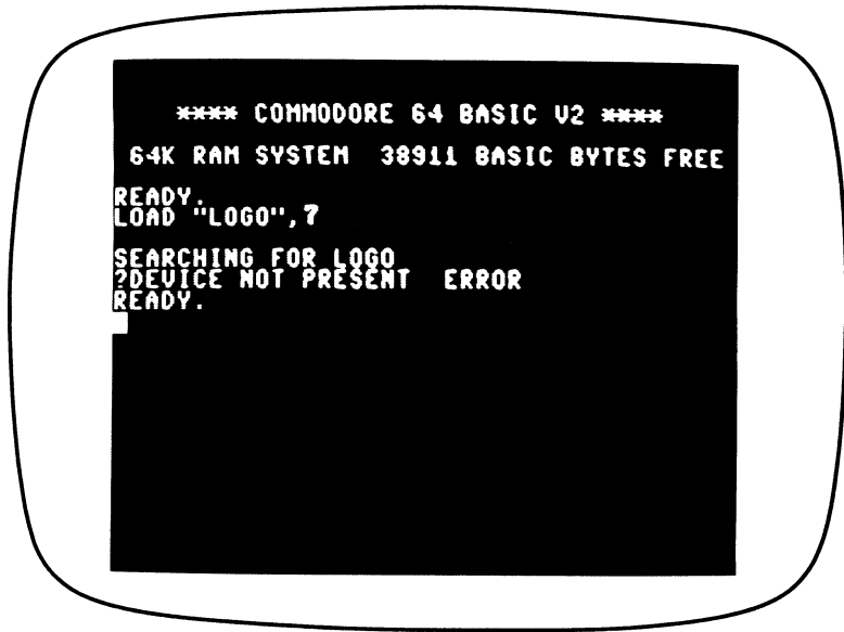
Figure 2-5. An error message appears on the screen when you type the wrong number in the LOAD command.
