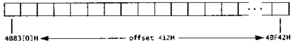
**Base Pointer (BP) register.** The 16-bit BP facilitates referencing parameters, which are data and addresses that a program passes via the stack. The processor combines the address in the SS with the offset in the BP. The 80386 and later processors have an extended 32-bit BP called the EBP register.
