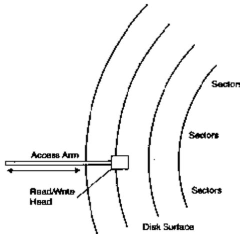
Figure 16-1 Disk Surface and Read/Write Head
