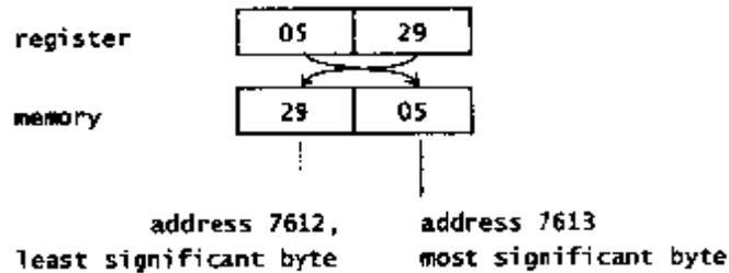
The processor expects numeric data in memory to be in reverse-byte sequence and processes the data accordingly. When the processor retrieves the word from memory, it again reverses the bytes, restoring them correctly in the register as hex 05 29. Although this feature is entirely automatic, you have to be alert to it when programming and debugging assembly language programs.
