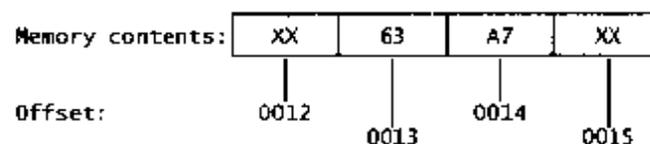
In this case, the processor has to perform two accesses. First, it accesses the bytes at 0012H and 0013H and delivers the byte from 0013H (63) to the AL register. Then, it accesses the bytes at 0014H and 0015H and delivers the byte from 0014H (A7) to the AH register. The AX now contains A763H.
