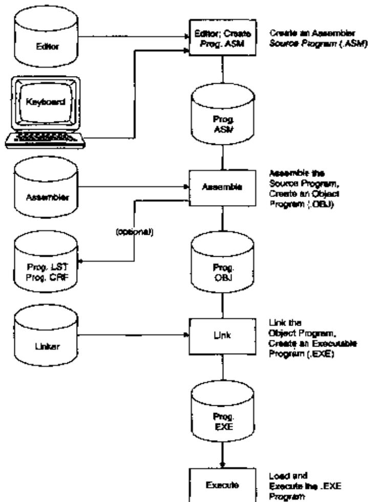
Figure 5-1 Steps in Assembly, Link, and Execute
