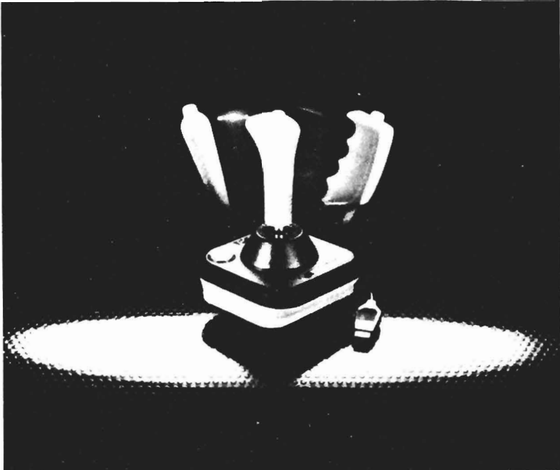
Figure 11.3 The WICO joystick has three different handles.
