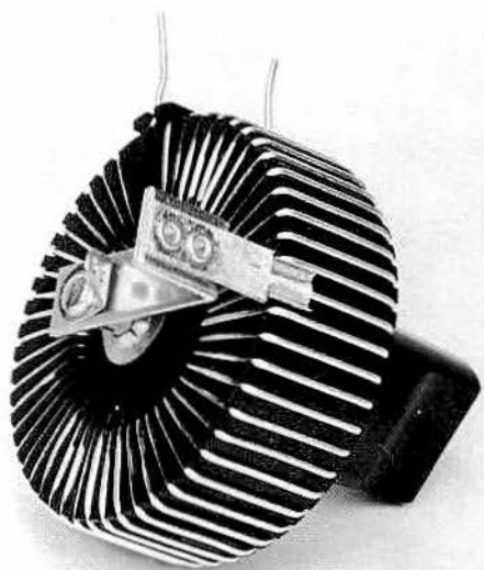
Figure 3-25 Commercially made toroidal type of variable inductor. This unit is manufactured by Ten Tec Corp. for use in their antenna Transmatch. The wiper is built so that it contacts one wire turn at a time, thereby preventing the shorted-turn effect.
