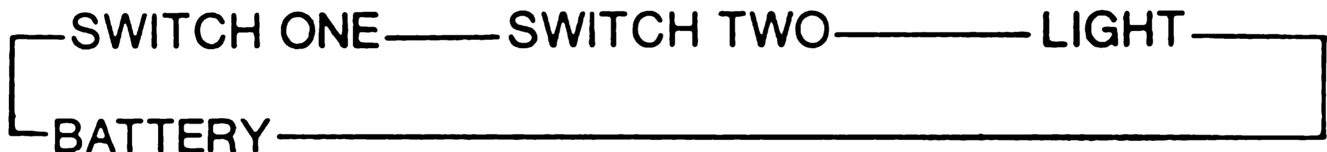
With both switches closed (that is, turned on, with their states **both** equal to 1 [1 1]) the light will glow. If **either** of the switches is off (one switch set to 1, and the other to 0 [1 0]) or both of them are off (switch one set to 0 and switch two equals 0 [0 0]) the light will be off. This is called an **AND** gate circuit.
