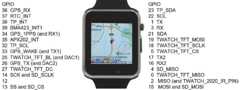
Figure 1-9. TTGO T-Watch V2 pin layout
