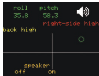
Figure 1-12. Digital spirit level
