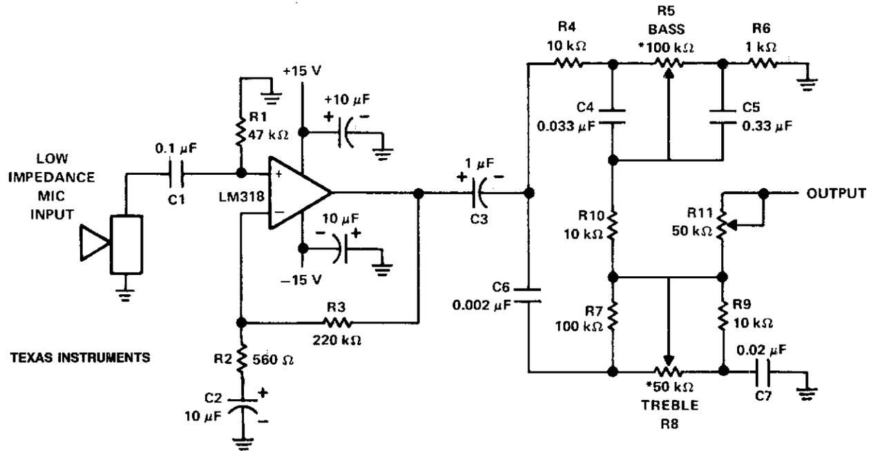
\*THE TONE CONTROLS ARE AUDIO TAPER (LOG) POTENTIOMETERS.
