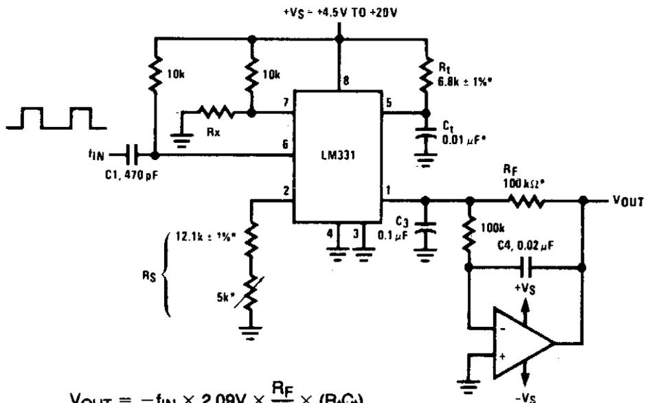
$$V_{OUT} = -f_{IN} \times 2.09V \times \frac{R_F}{R_S} \times (R_T C_T)$$
