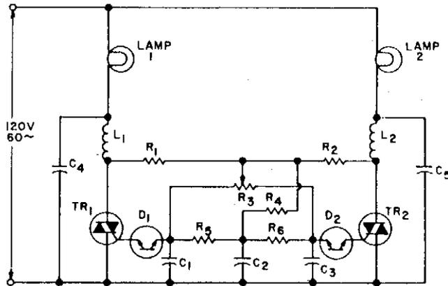
$R_1 = R_2 = 6800\Omega$ , 1WATT
