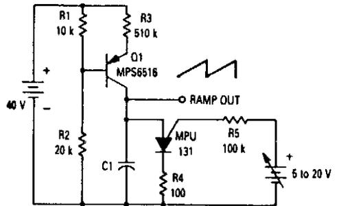
**Voltage Controlled Ramp Generator (VCRG)**
