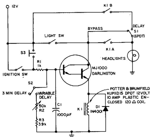
1. Automobile headlights may be kept on up to 3 minutes after you leave the car with this Darlington time-delay circuit.
