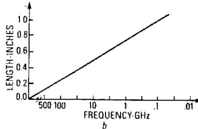
FIG. 3—VARY THE LEAD LENGTHS OF C1 to tune the input circuit.
