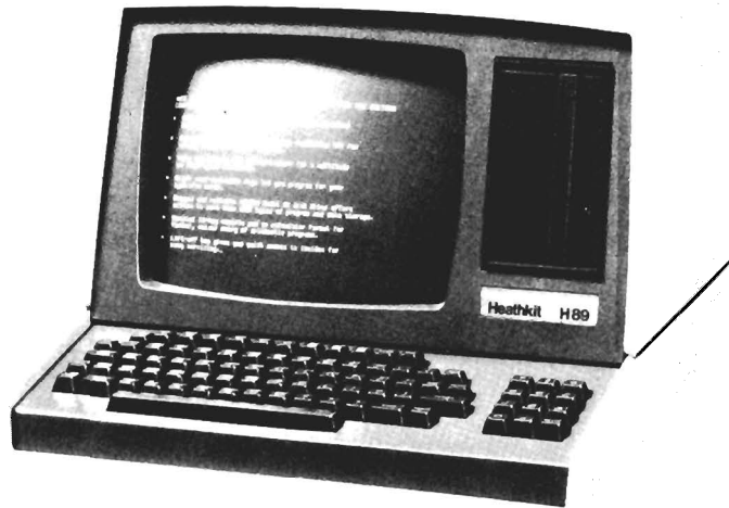
Figure 1-1 New Heathkit H89 All-In-One Computer features two Z80 processors, floppy disk storage, smart video terminal, heavy-duty keyboard, numeric keypad and 16K RAM, all in one compact unit. (Courtesy of Heath/Zenith)
