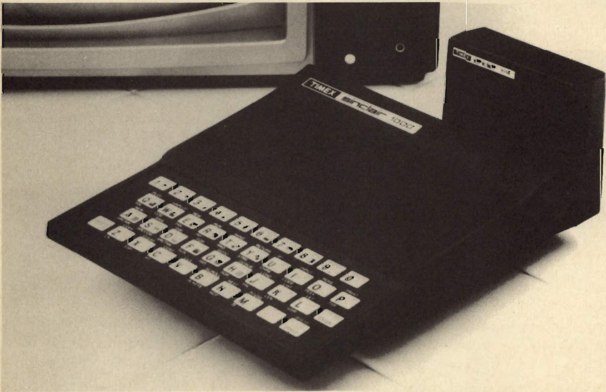
The Timex/Sinclair 1000 is a true low-cost computer. It's also powerful, and it has moving graphics, single-key entry, mathematical functions, and error detection. It hooks up to a home television set.
