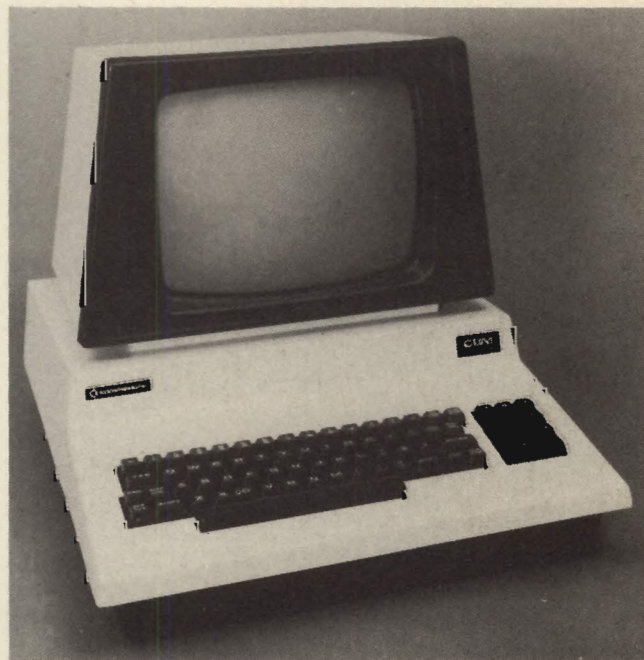
The Commodore CBM, designed for small business use, displays a full 80-character line on its screen.
