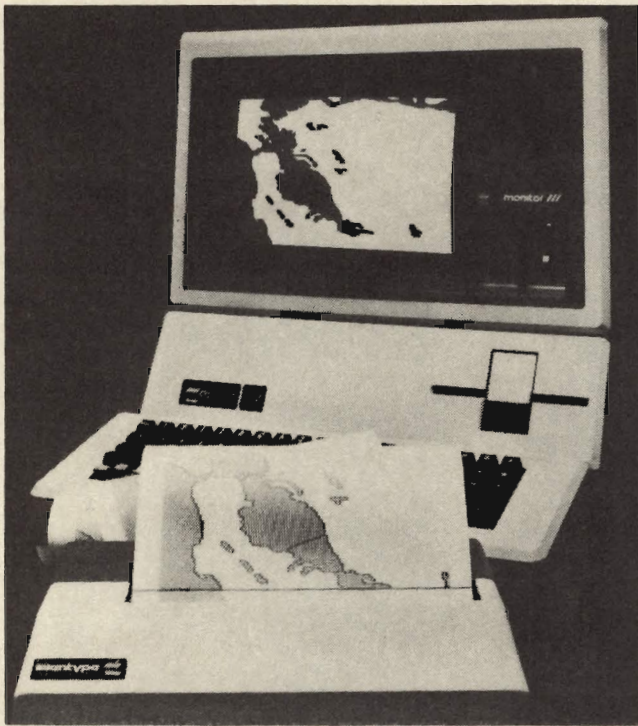
Some printers can produce charts, graphs, and other images off the computer's video display screen.
