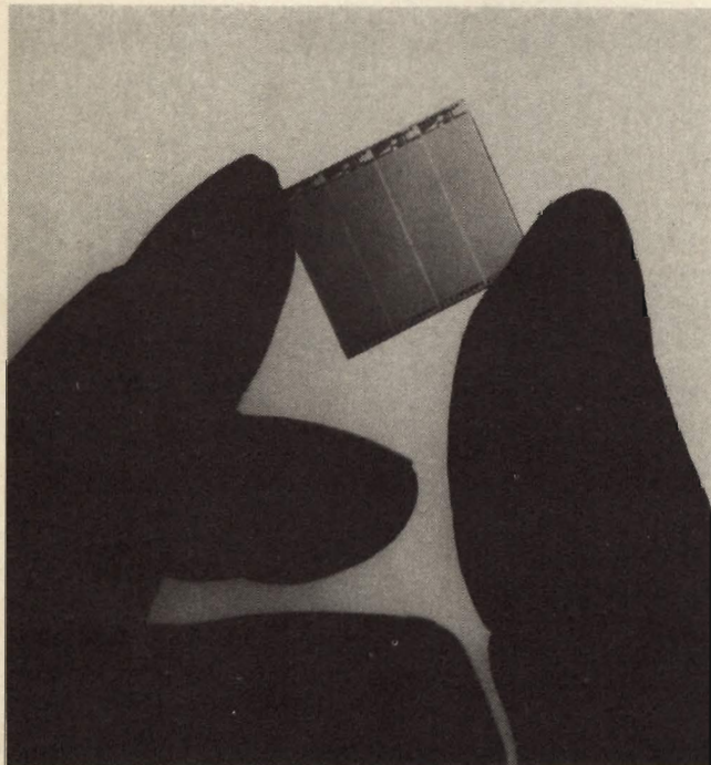
Bubble memory cartridges can store huge amounts of data, in microscopic magnetic bubbles.
