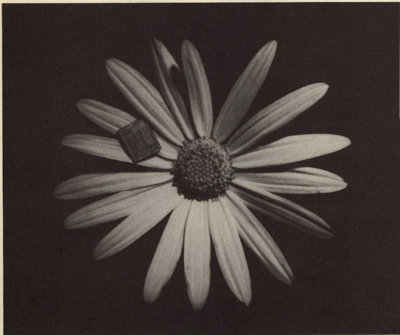
The microprocessor chip, so tiny it's dwarfed by a daisy, is the real brains of the computer. It's made of silicon, and etched with thousands of electronic circuits—the transistors that actually do the computing.
