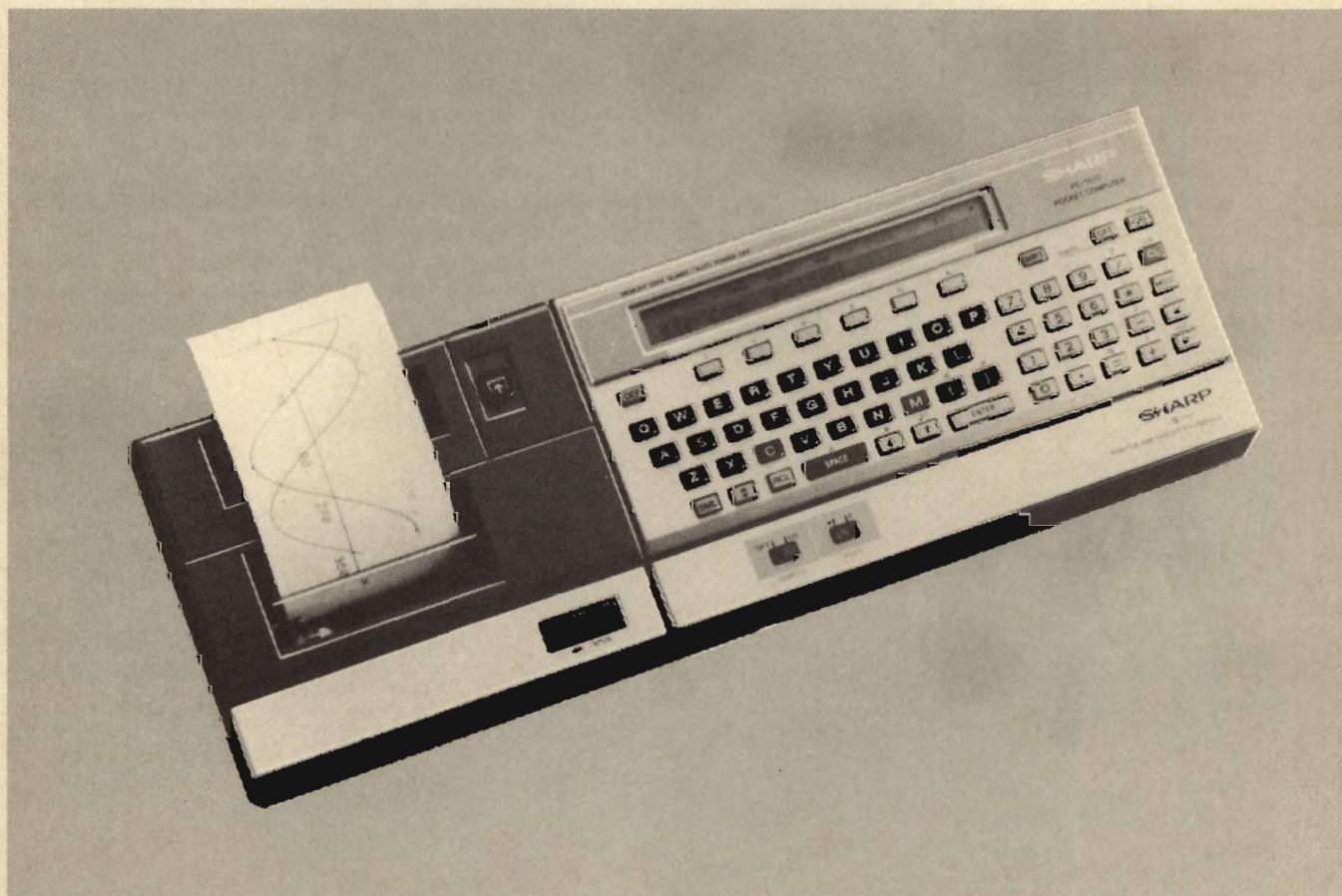
The Sharp PC-1500, with the same capabilities as the TRS-80 PC-2, is far from being a glorified calculator. One exciting accessory is a printer, which produces printed characters, graphs, and even drawings.
