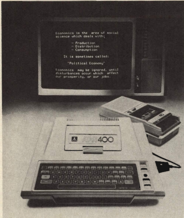
The Atari 400 has 16K of RAM, and can handle the full range of Atari software on cassettes and cartridges.
