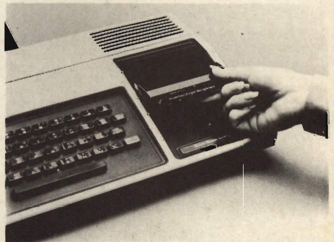
The TI 99/4A is primarily designed to be used with plug-in cartridges called "Command Modules."
