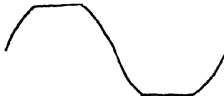
This is a sine wave with its peaks flattened (or cut off). It causes distortion, harshness, and trouble. A telephone earpiece has a dual diode connected across the terminals in newer units, and if the signal level is too great the diodes absorb the peaks of the sine wave, thus causing the waveform to distort like this. Remove the diode before using.
