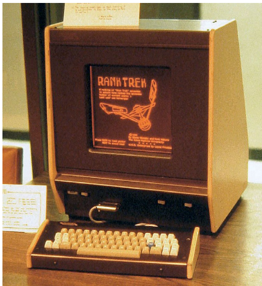
A PLATO terminal, with its distinct orange plasma display. By 1976 there were 950 of these terminals across the globe.
