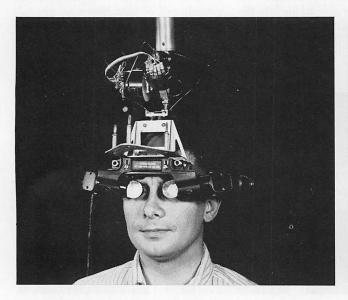
HEAD-MOUNTED DISPLAY at the University of Utah employs a display processor similar to that used for the aircraft carrier sequence. Two miniature cathode ray tubes are built into the goggles. A mechanical linkage tells the computer where the viewer is tooking at each instant. The display processor instantaneously surplies
