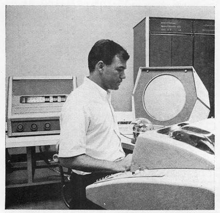
ANOTHER TERMINAL is the "Kluge" display system developed by M.I.T.'s Electronic Systems Laboratory. It has a control unit, display screen, light pen and other equipment.
