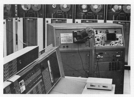
COMPUTER AND SCANNING DEVICE used by the authors are located at the Goddard Space Flight Center outside Washington, D.C. The IBM 7094 computer (foreground) receives descriptions of photomicrographs of chromosomes from the fidac scanner (background), on the basis of which it counts, analyzes and collates data on the chromosomes.
