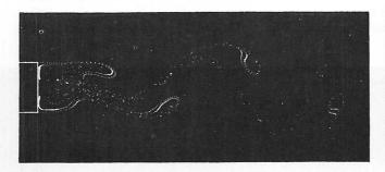
STREAK-LINE PLOT is a third kind of configuration possible in computer experiments. In this case, indicator numbers that do not play any part in the flow calculations have been inserted in four cells of the computer mesh at the rear of the obstacle. These numbers become "computational particles" that trace out the downwind eddies in streaks, as do smoke filaments in a wind tunnel.
