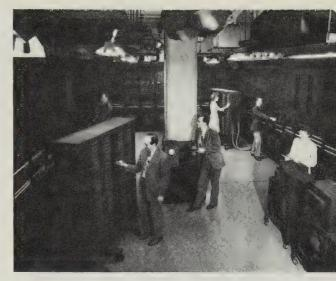
This photo shows the ENIAC, the first electronic computer, in operation.
