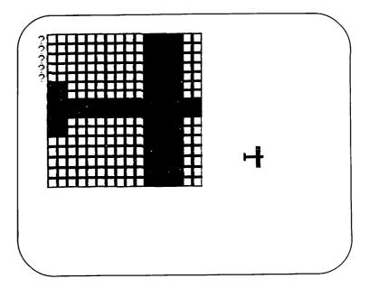
As you can see from the figure, large and small images of the plane both appear on the screen at the same time. If you count the boxes in the large grid, you will see that sprite shapes are made from larger matrices than those for tiles. Character tiles are formed from  $8\times 8$  dot arrays, whereas sprite shapes are formed from  $16\times 16$  dot arrays.
