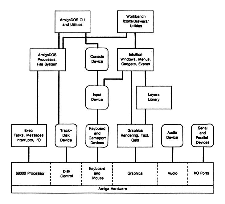
Figure P-1: Amiga System Software Modules
