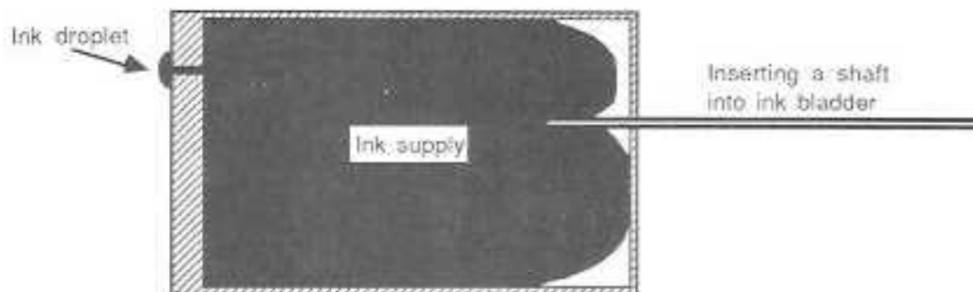
Fig. 9-7. Clearing replaceable ink jets.
