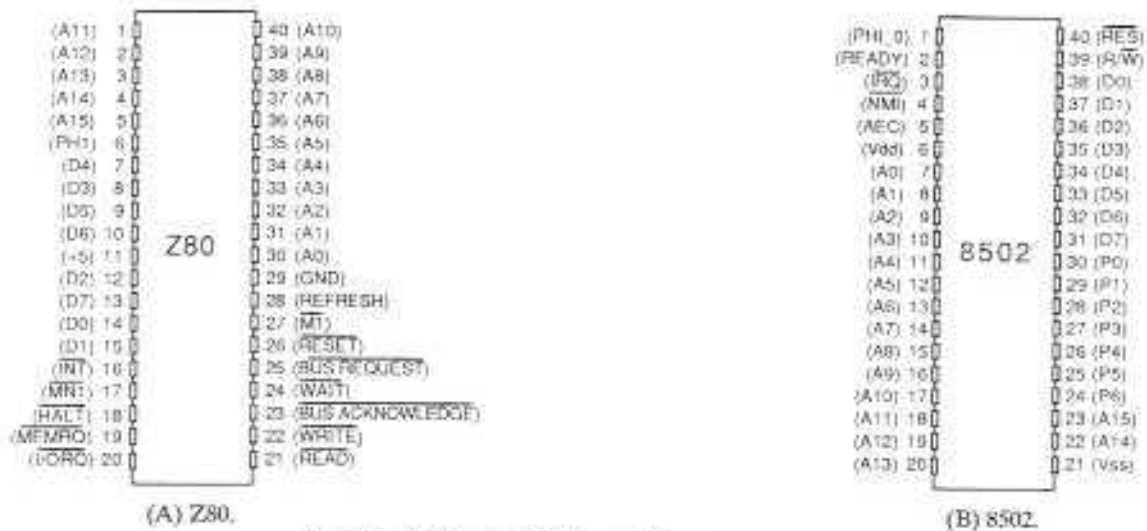
Fig. 2-8. 8502 and Z80 pinout diagram.
