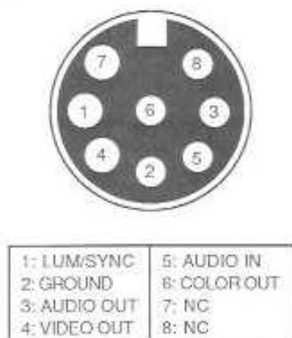
Fig. 6-1. Composite video cable connector and pinouts.
