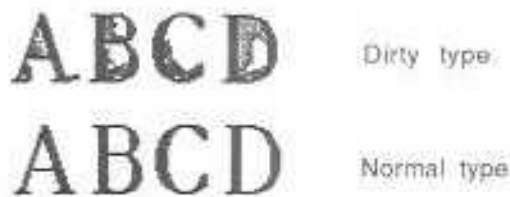
Fig. 9-5. Filled characters produced by a dirty printwheel.
