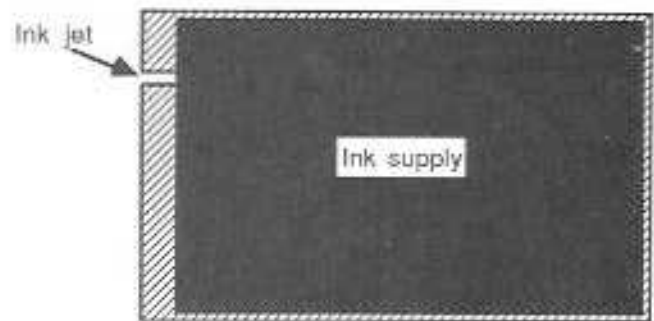
Fig. 9-6. Cross section of an ink jet head.
