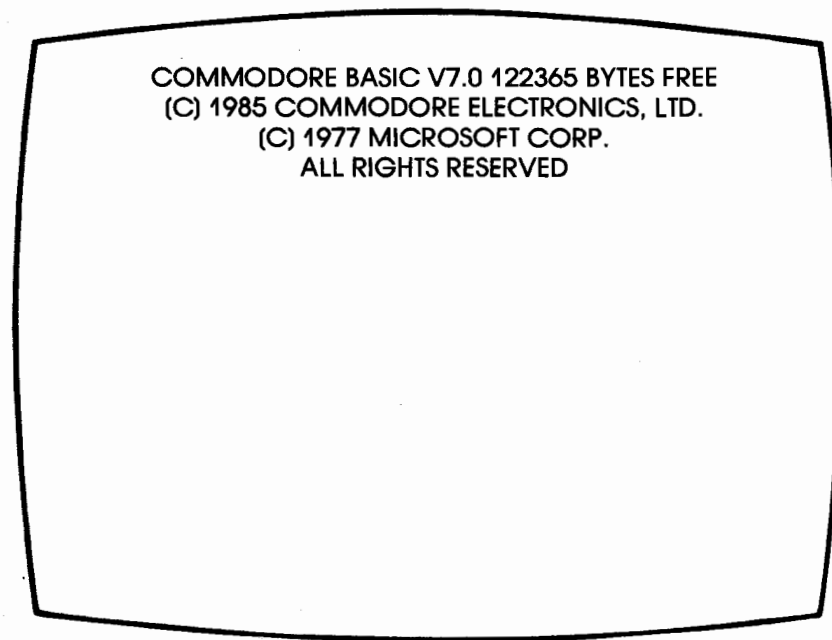
Fig. 1-2 Heading message that appears when system is first set to C128 mode. Border and characters are light green and background is dark gray
