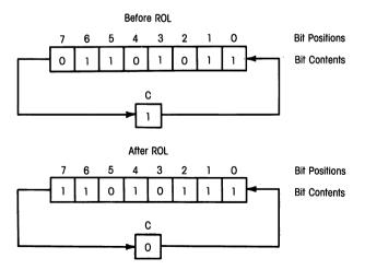
ROL, like ASL, can be used to shift the contents of the accumulator or a memory register one place to the left. But ROL does not place a 0 in the bit 0 position. Instead, it rotates the carry bit into bit 0
