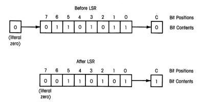
LSR, like ASL, works on whatever binary number is in the 8502's accumulator. But LSR shifts each bit in the number one position to the right. Bit 7 of the new number, left empty by the LSR instruction, is filled with a 0. And the LSB (least significant bit), bit 0, is put into the carry flag of the P register.
