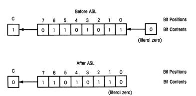
As figure 8-1 illustrates, the ASL instruction moves each bit in an 8-bit number one space to the left—each bit, that is, except bit 7. Bit 7 drops into the carry bit of the processor status register. Bit 0 of the new number, left empty by the ASL instruction, is filled with a 0.
