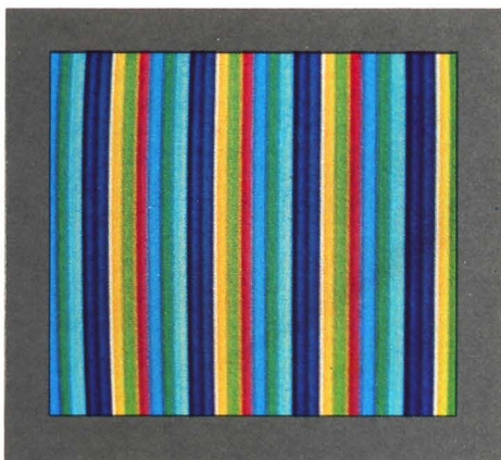
1 SEMIGRAPHIC 4 MODE An example of the Color BASIC mode of 64 pixels horizontally by 32 pixels vertically, this photograph shows available colors. (Chapter 1)
