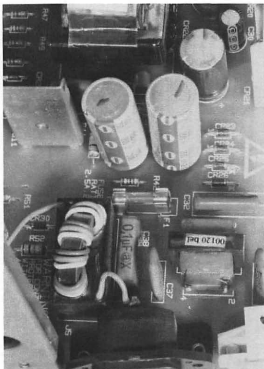
FIG. 6-2 Checking the fuse can be done visually. Better yet, use your VOM and test for continuity.
