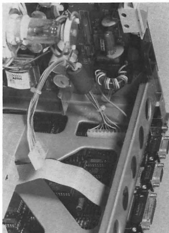
FIG. 6-14 The 10-pin power supply connector is the white plug near the center of the photograph.
