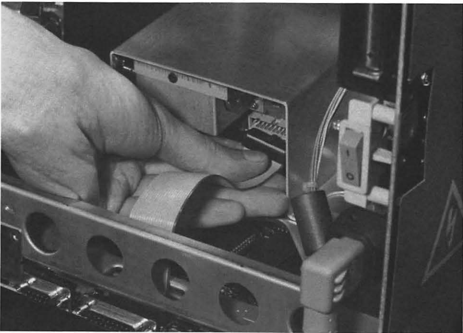
FIG. 4-20 Disconnect internal drive and move cable to the back of the computer.
