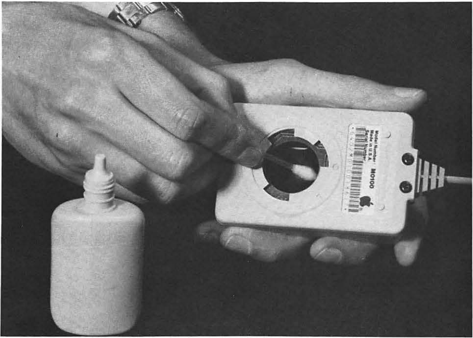
FIG. 6-38 When cleaning the chamber, use a tight swab and a high quality cleaner.
