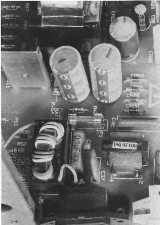
FIG. 1-2 There are 120 deadly volts passing through that fuse when the power is on.
