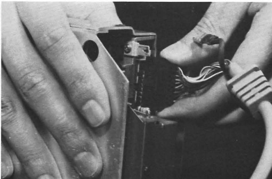
FIG. 4-18 Even more carefully, unplug the cable.
