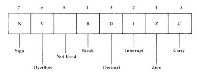
The bits of the Status Register are numbered from right to left, 0–7. Each bit in this register indicates the status and/or results of different operations and is called a flag. It is by using this register that we can create counters and loops in our programs. The flag we will be immediately concerned with is bit one, the *zero flag*. In terms of the commands we already know, the zero flag is affected by an LDA, LDX, or LDY.
