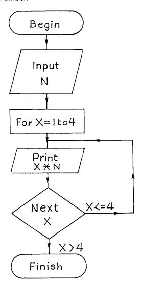
10 INPUT N 20 FOR X = 1 TO 4 30 PRINT X \* N 40 NEXT X Each time the conditional symbol is reached, X is incremented and a decision is made based on its new value. If X is 4 or less, the loop continues and another result is printed; if X exceeds 4, the run ends. The two exit symbols from the conditional allow these two possibilities.
