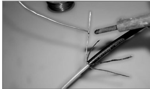
Figure 8 Cover the bundles with solder. Although this step is optional, it does enable the ground plane elements to hold their shape better, and prevents untwisting of the strands.
