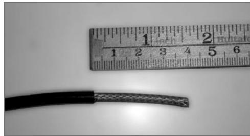
Figure 2 Cut off about 40 mm of the outer insulation. This will expose the braid that forms the cable shield.
