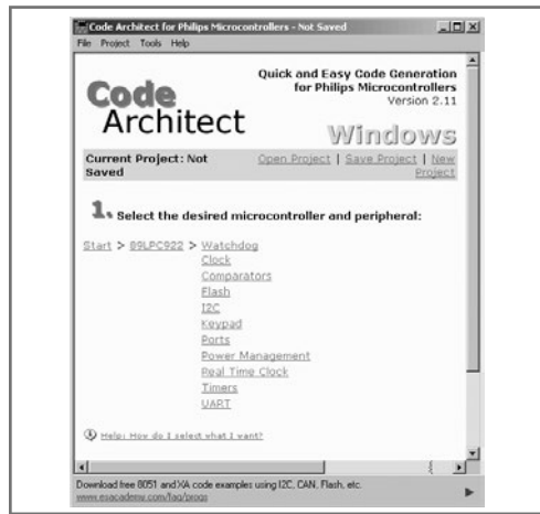
Figure 1 'Code Architect' is a free tool that makes using the LPC900 microcontroller very straightforward.
