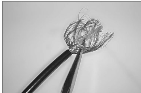
Figure 4 Using the pointed tool, carefully unweave the braid strands.
