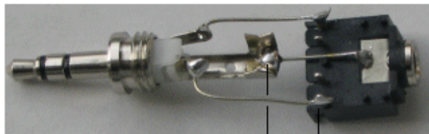
Above: A 3.5mm switched stereo plug and socket wiring.
